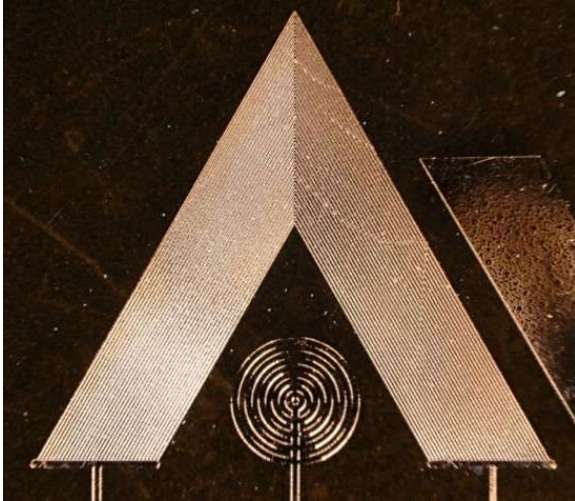
25 \mu\text{m} line & space by full additive process
