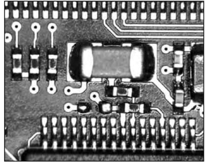
*Surface mount passive components, large and small (center and adjacent)*
