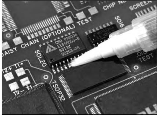
*Rework of gull-wing leaded SMDs: applying liquid flux prior to heating. Components in foreground have "fine pitch" lead spacing.*
