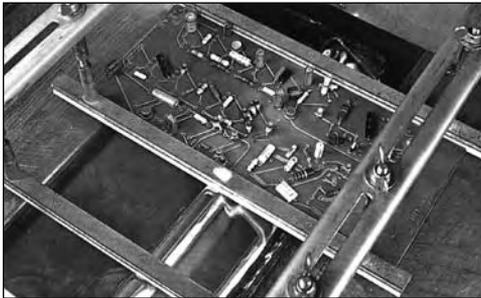
*Early wave soldering of a through hole demo board, late 1960s*
