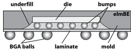
The flip-chip concept is not new, having been around as early as the 1960s when IBM used them for their mainframes. Since then, various companies have developed the flip-chip for use in thousands of different applications, taking advantage of the size and cost benefits offered by this assembly method. Flip chips have likewise eliminated performance problems related to inductance and capacitance associated with bond wires.
