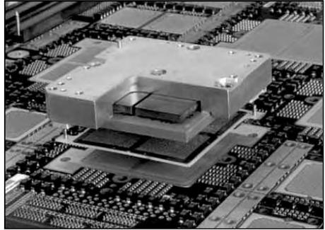
*The DataStar Supercomputing cluster at the San Diego Supercomputer Center has 2464 processors and is the 35th most powerful supercomputer in the world. One DataStar node, the IBM p655+, employs an 8-processor Power4+ -based multichip module (shown above), that consists of four integrated dual-core chips.*
