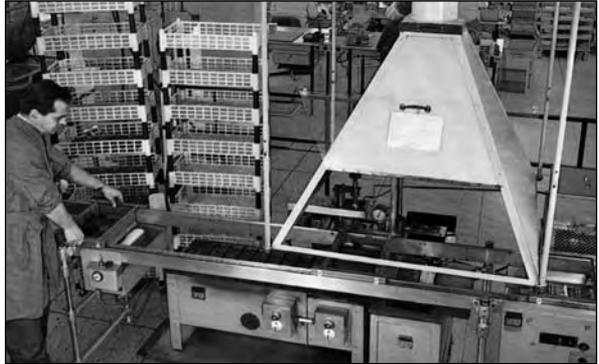
*Horizontal production wave soldering machine, mid-1960s*
