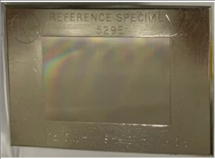
Representative 3D laser images of the Rubert roughness standard, model KB-RS529.
