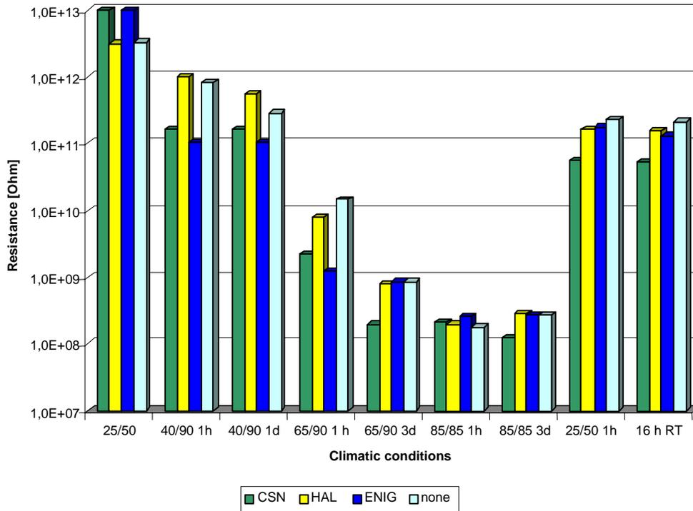
**Figure 7 - Insulation resistances of a photoimageable solder mask with different surface finishes after a thermal cycling test (1,000 cycles, -40°C [-40°F] / +150°C [302°F])**
