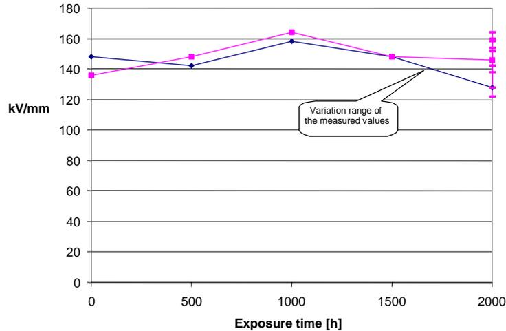
**Figure 6 - Tracking resistance (CTI) of a photoimageable solder mask after long-term thermal storage at 150°C [302°F]**
