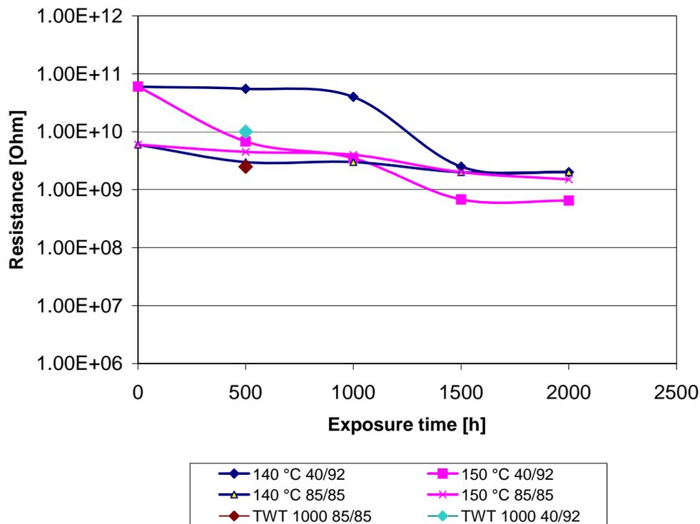
**Figure 8 - Correlation of the insulation resistance of a photoimageable solder mask after continuous thermal storage at 140 and 150°C [284 and 302°F] and the corresponding time in the thermal cycling test (-40°C [-40°F]/+150°C [302°F]) (TCT)**
