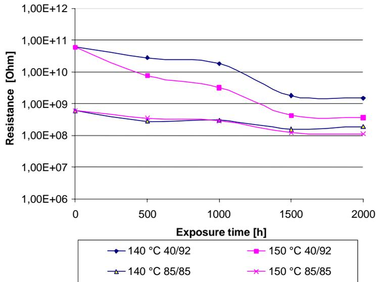
**Figure 3 - Insulating resistances of a photoimageable solder mask after long-term thermal storage at 140°C [284°F] and 150°C [302°F]**
