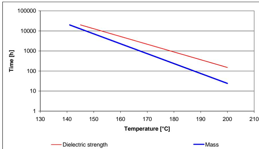
**Figure 2 - Graph showing the extrapolation of the failure times determined in appropriate tests over a failure period of 20,000 hours**
