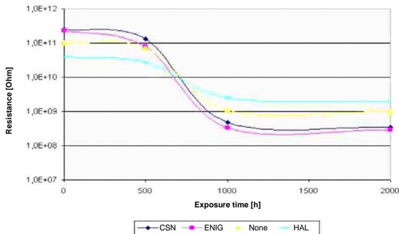
**Figure 4 - Insulating resistances of a photoimageable solder mask processed with various surface finishes after long-term thermal storage at 150°C [302°F] (Nickel/Gold finish [ENIG], chemical tin finish [CSN] and Hot-Air Levelling [HAL]; 40°C [104°F]/92% r. h.)**
