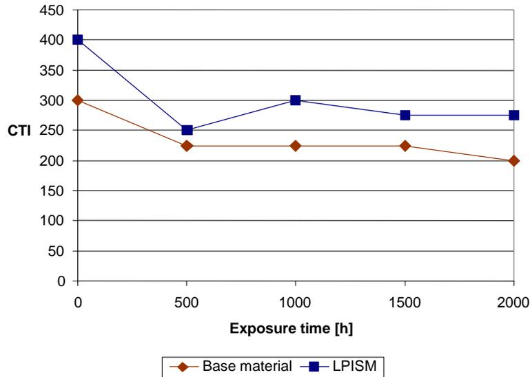
**Figure 5 - Tracking resistance (CTI) of a photoimageable solder mask after long-term thermal storage at 150°C [302°F]**
