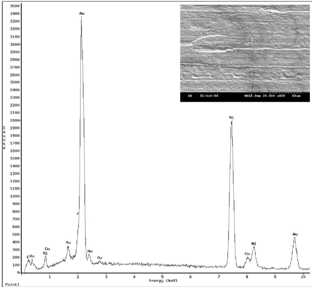
**Figure 1 - SEM micrograph and EDX spectrum of IG over low phosphorus EN panel. Inset SEM micrograph shows porosity in the IG surface, 600X.**
