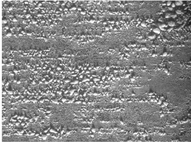
**Figure 12 - Photomicrograph of sulfur dioxide porosity tested surface of IG over high phosphorus EN panel, 10X.**
