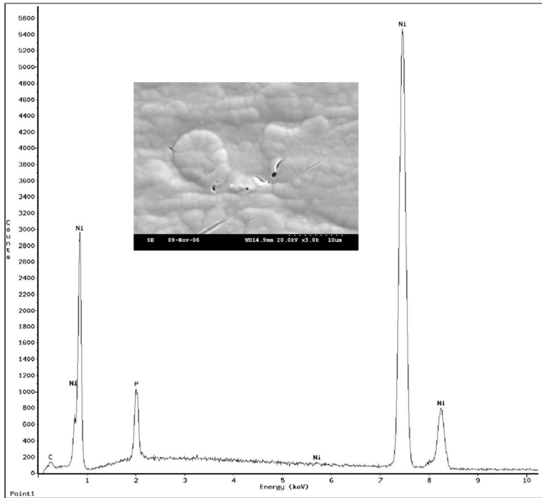
**Figure 5 - SEM micrograph and EDX spectrum medium phosphorus EN panel. Inset SEM micrograph shows porosity in the EN surface, 3000X.**
