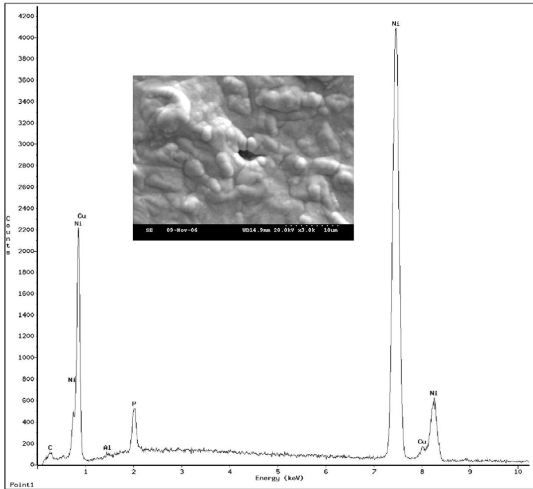
Figure 4 - SEM micrograph and EDX spectrum low phosphorus EN panel. Inset SEM micrograph shows porosity in the EN surface, 3000X.
