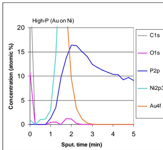
**Figure 9 - XPS depth profile plot of IG over medium phosphorus EN panel showing undetectable levels of oxygen and carbon at the gold-nickel interface and in the bulk EN.**
