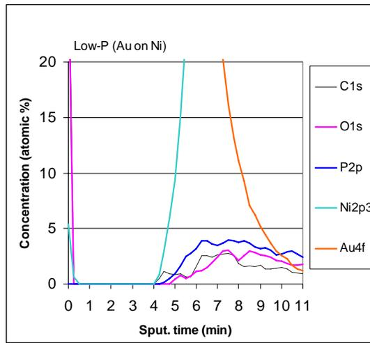
**Figure 7 – XPS depth profile plot of IG over low phosphorus EN panel showing presence of oxygen and carbon at and below the gold-nickel interface.**
