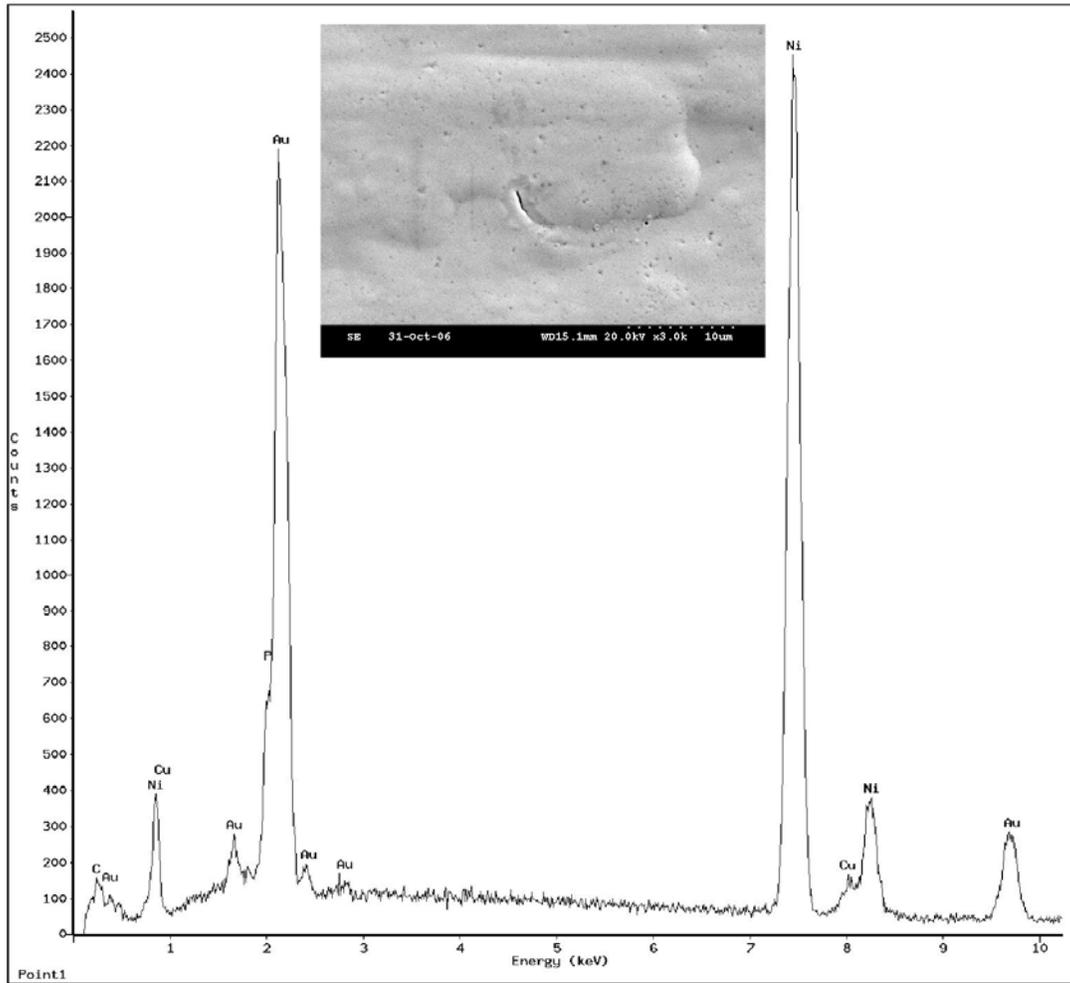
**Figure 2 - SEM micrograph and EDX spectrum of IG over medium phosphorus EN panel. Inset SEM micrograph shows porosity in the IG surface, 3000X.**
