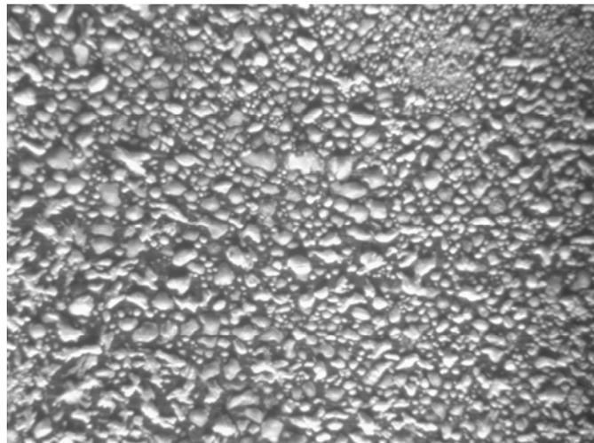
**Figure 10 - Photomicrograph of sulfur dioxide porosity tested surface of IG over low phosphorus EN panel, 10X.**
