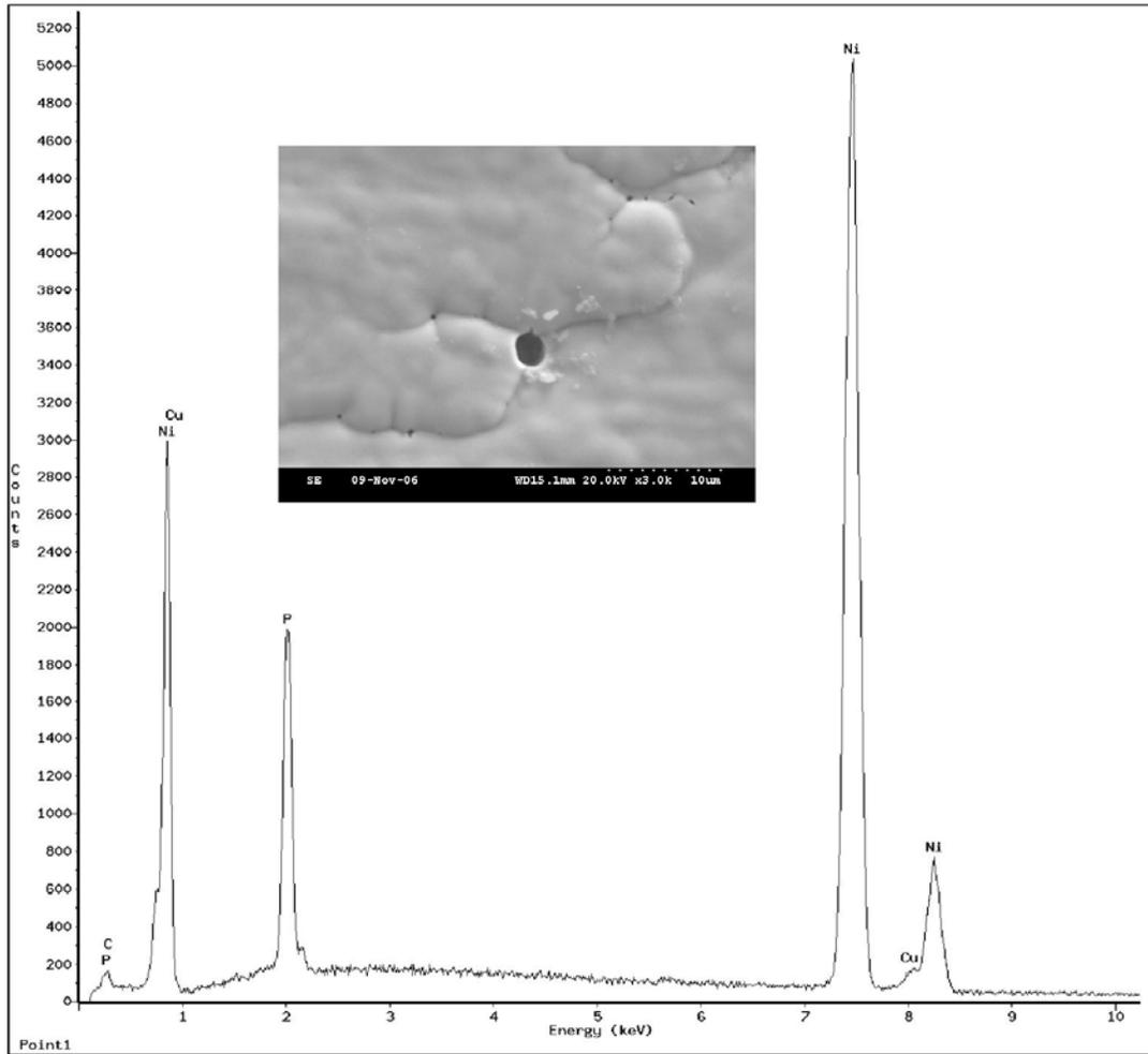
Figure 6 - SEM micrograph and EDX spectrum high phosphorus EN panel. Inset SEM micrograph shows porosity in the EN surface, 3000X.
