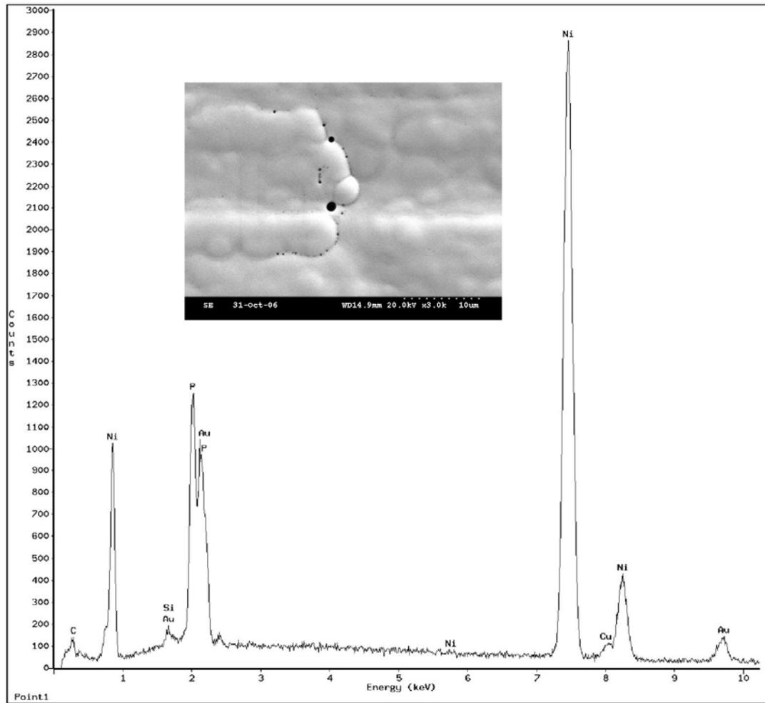
**Figure 3 - SEM micrograph and EDX spectrum of IG over high phosphorus EN panel. Inset SEM micrograph shows porosity in the IG surface, 3000X.**
