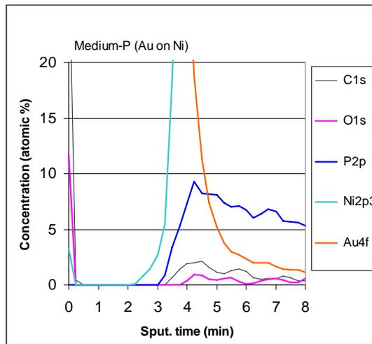
**Figure 8 - XPS depth profile plot of IG over medium phosphorus EN panel showing presence of oxygen and carbon at and below the gold-nickel interface.**
