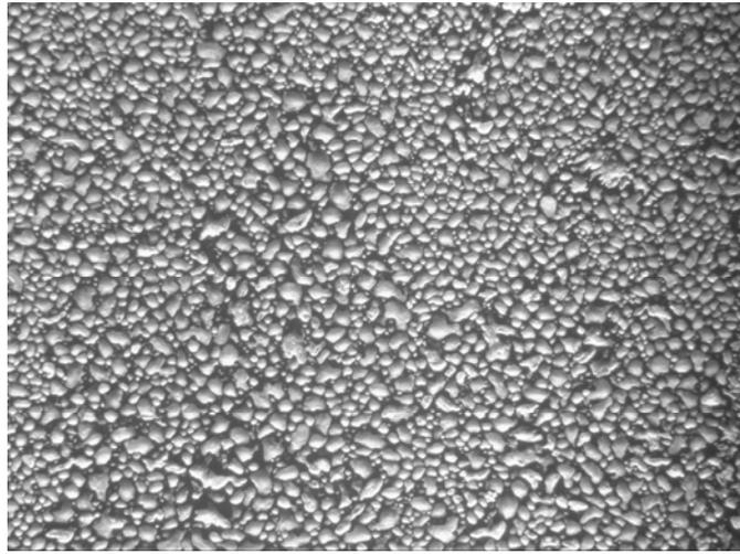
**Figure 11 - Photomicrograph of sulfur dioxide porosity tested surface of IG over medium phosphorus EN panel, 10X.**
