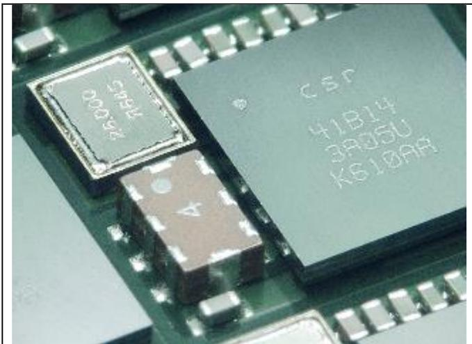
**Figure 1 - Highly Dense Circuit Assembly**
