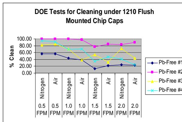
**Figure 8 - 1210 Cleaning Data from Spray Manifold #2**
