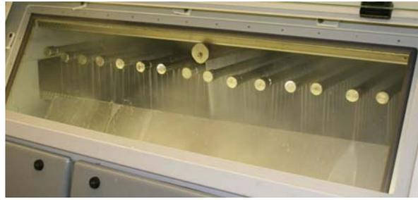
**Figure 10 - Wash Spray Manifold #3**
