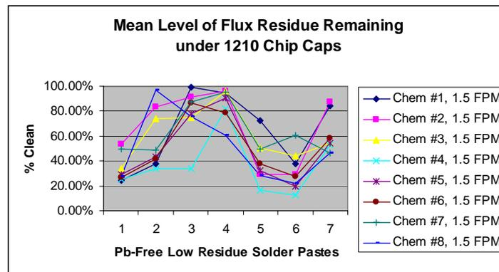
**Figure 6 - Cleaning Data from Wash Spray Manifold #1**
