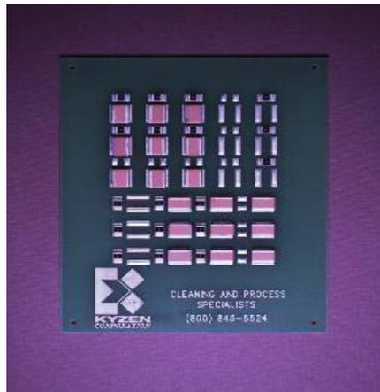
**Figure 2 - Test Board Design**
