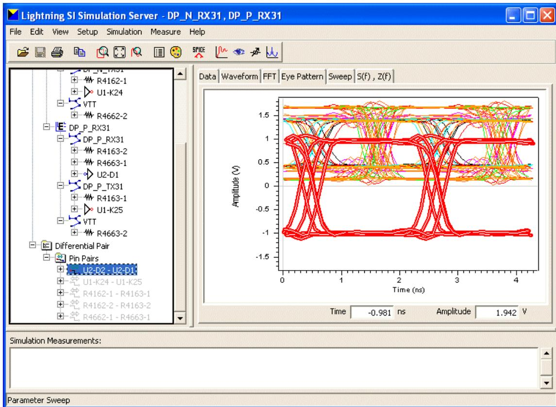
**Eye diagram for the routed differential pair showing good comparison with the eye diagram simulated in the pre-design scenario**
