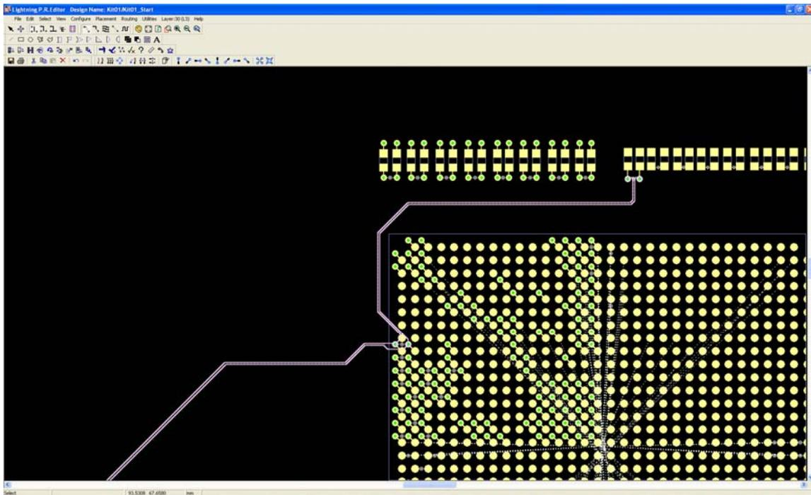
**The Differential Pair, Routed to SSTL Class I Topology Constraints**
