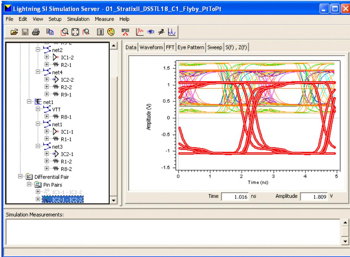
**Eye diagram obtained for the 1.8V Differential Class I SSTL signal**
