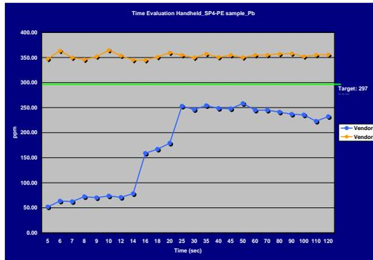
Figure 4 - The handheld XRF Pb element results for detection level versus acquisition time study
