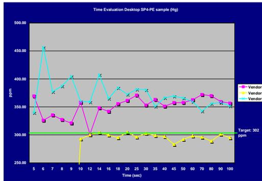
Figure 5 - The desk top XRF Hg element results for detection level versus acquisition time study
