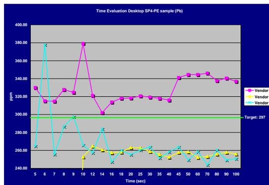
**Figure 3 - The desk top XRF Pb element results for detection level versus acquisition time study**
