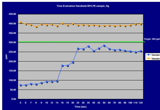
Figure 6 - The handheld XRF Hg element results for detection level versus acquisition time study
