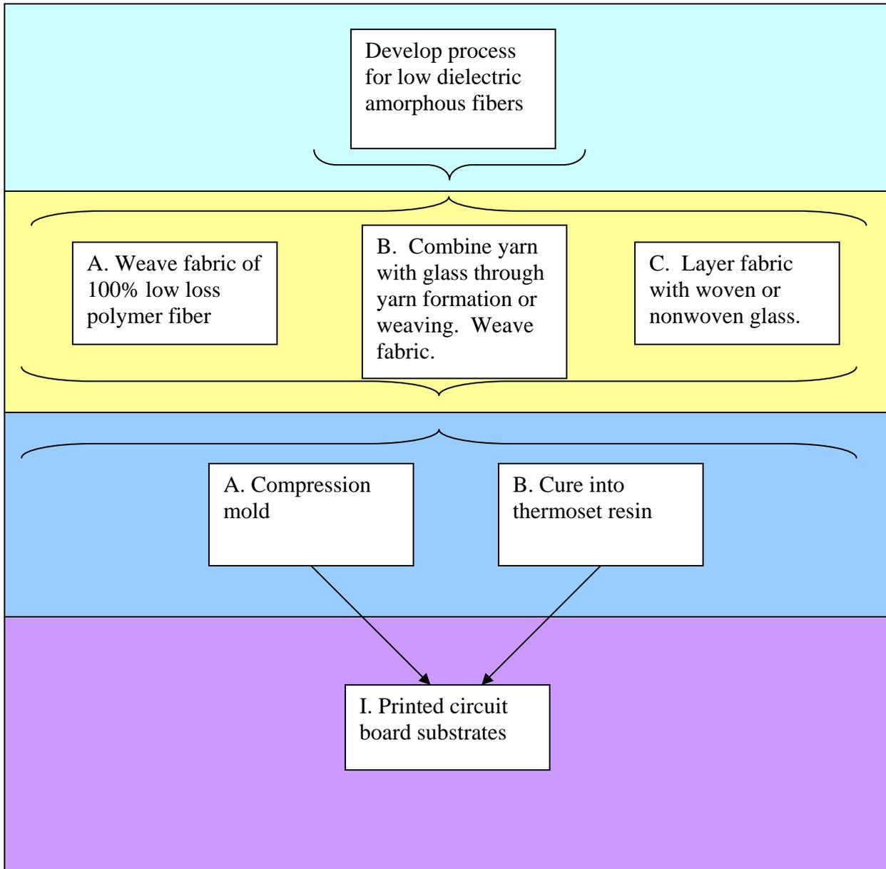
**Figure 1 - Ways of combining glass, low dielectric fibers, and resins to form affordable microwave circuit board substrate materials.**
