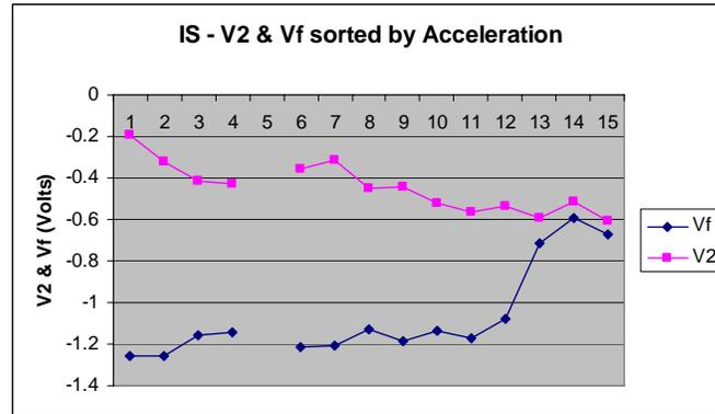
Figure 21 IS  $V_f$  and  $V_2$  Values Ordered Using Acceleration Equation
