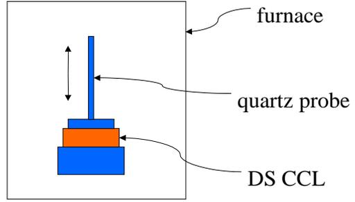
DS CCL – Double Sided Copper Clad Laminate, no copper removed
