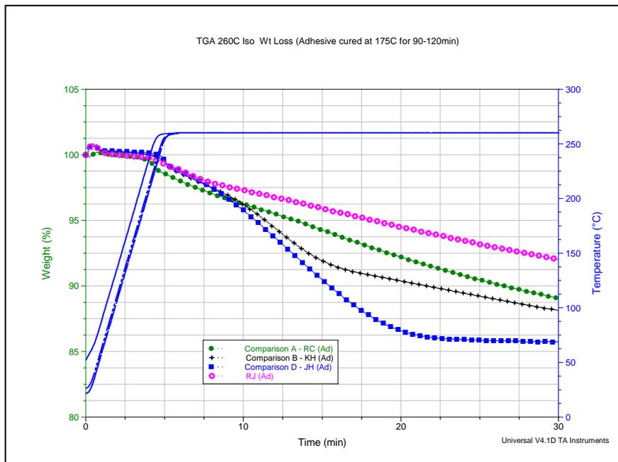
**Figure 2 - TGA Wt Loss at 260°C of Different Adhesive Systems**
