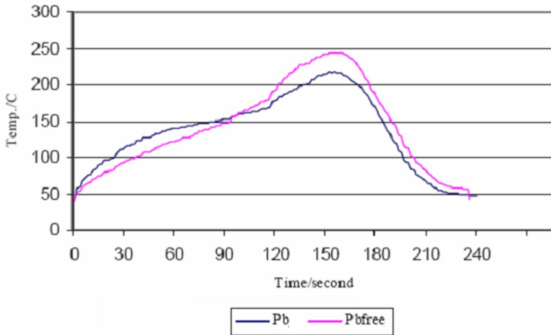
**Figure 7 - Typical Solder Reflow part temperature Profile for Eutectic (Pb) and Lead Free solder (Pbfree)**
