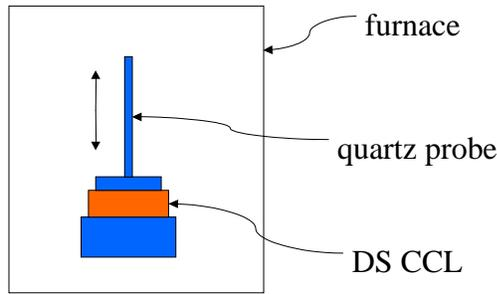
**Figure 3 - TMA probe and sample setup in the furnace.**
