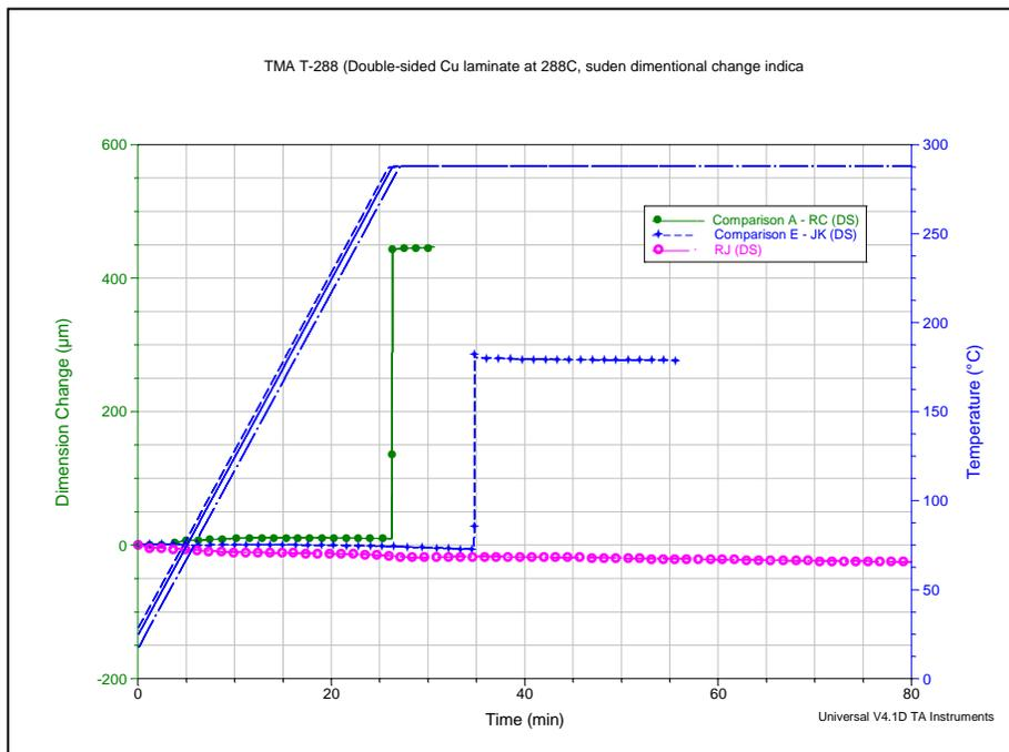
**Figure 4 - TMA T-288 Test Results of Different Adhesive Based Double sided Cu Clad Samples**
