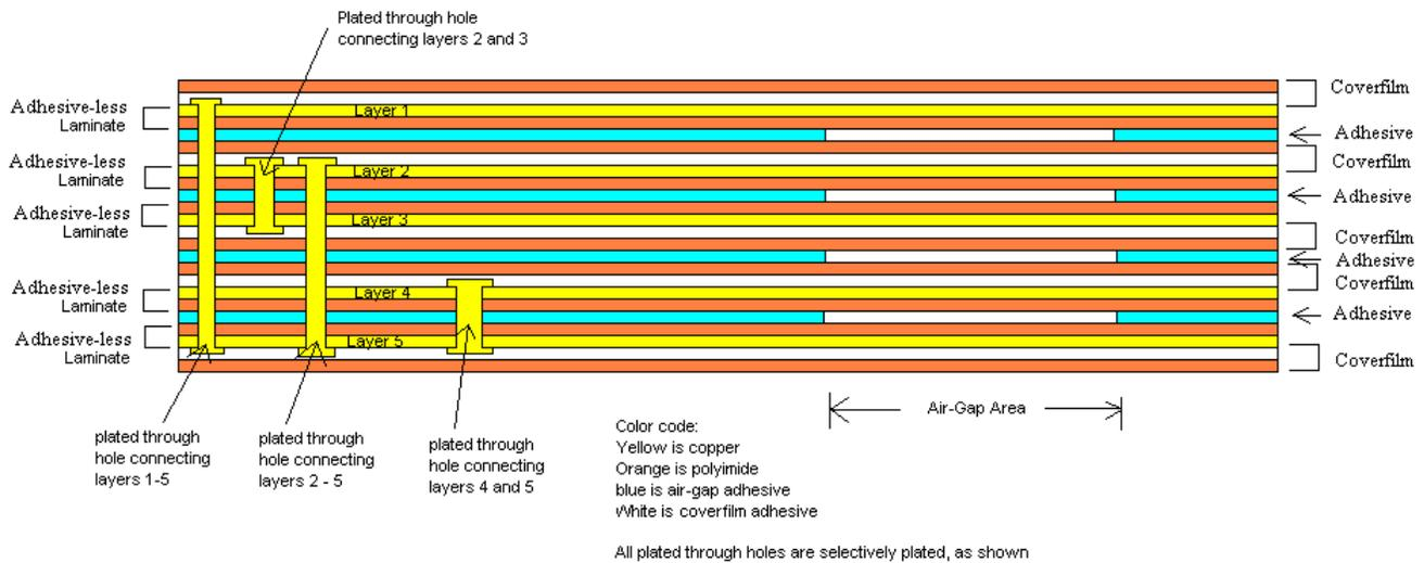
**Figures 6 - Cross-sectional view of a 5 layer cell phone hinge flex circuit**
