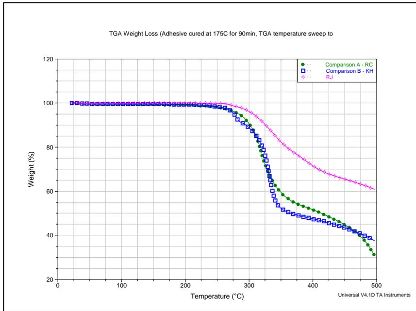
**Figure 1 - TGA Wt Loss During Heating of Different Adhesive Systems**
