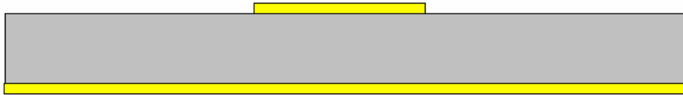
Figure 12, cross-sectional view of a high frequency double-sided circuit board
