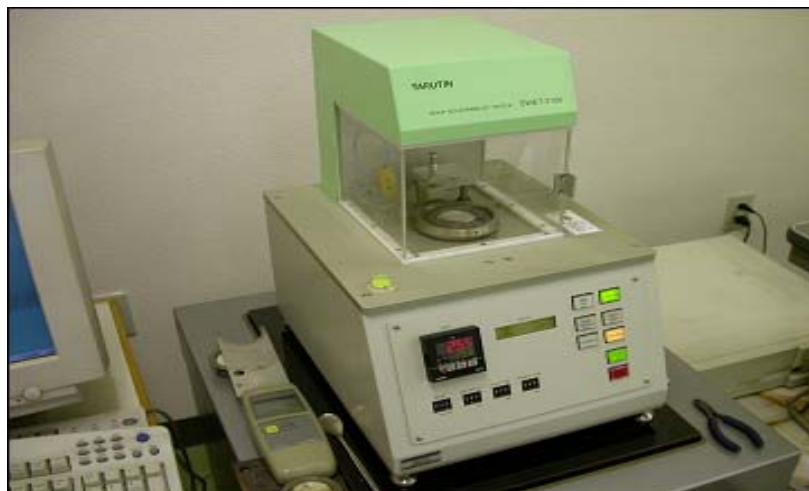
Figure 9. Wetting balance test apparatus
