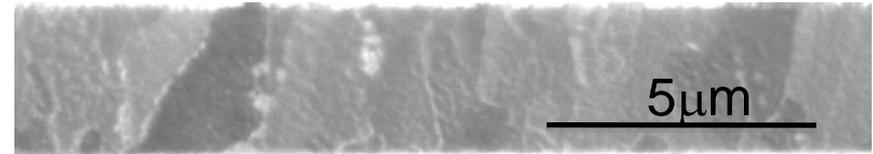
FIB cross section 4μm(above) and 12μm (below) thick film deposited from electrolyte ‘A’
