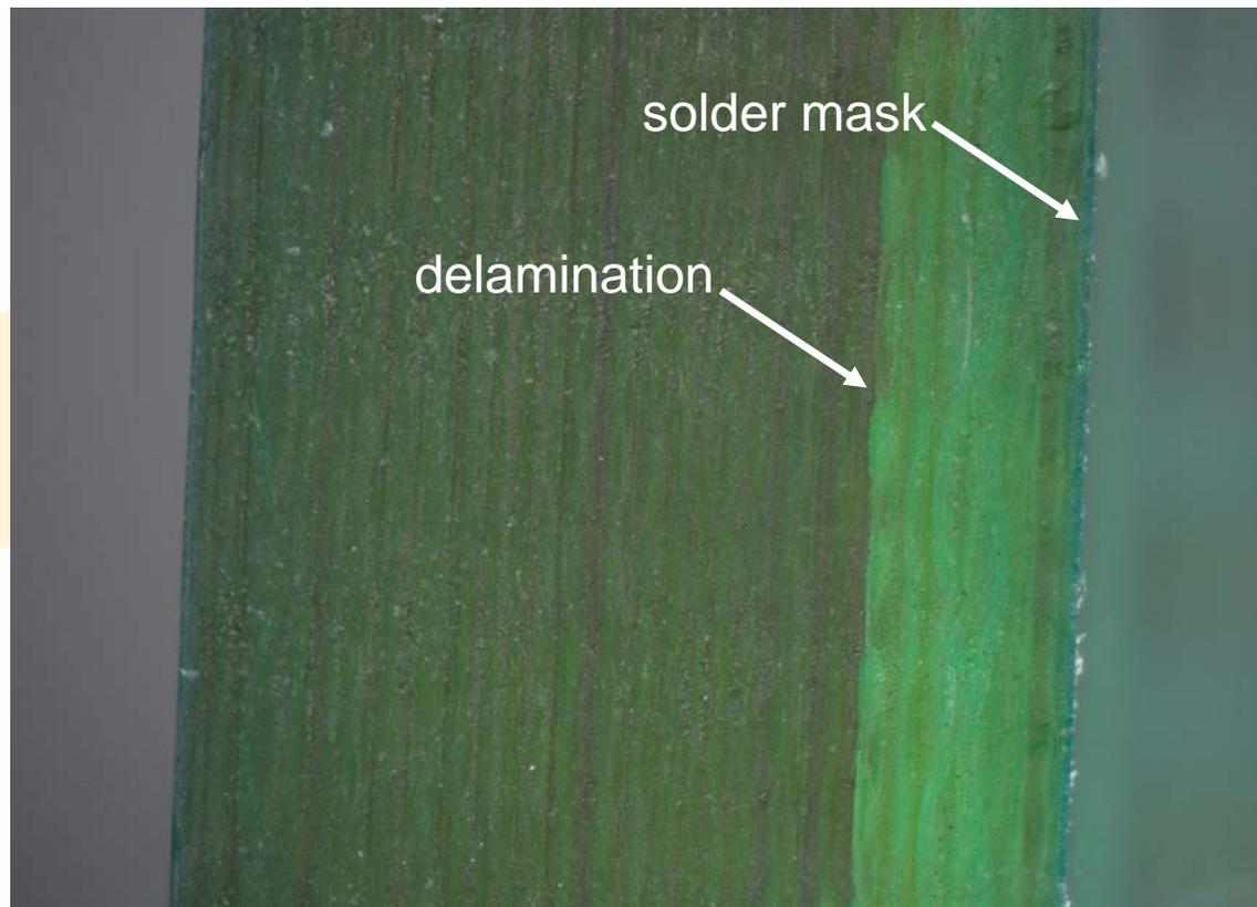
2.5X side view of 85°C/85%RH board after 3 reflows at 260°C peak
