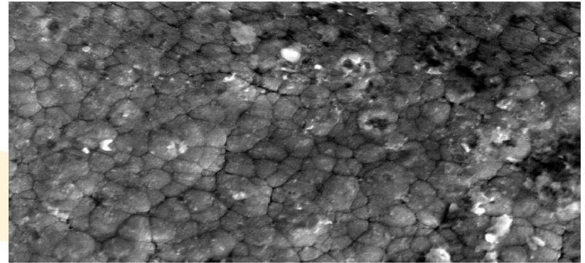
Figure 7. Higher magnification shows a pattern of deeply grooved grain boundaries.
