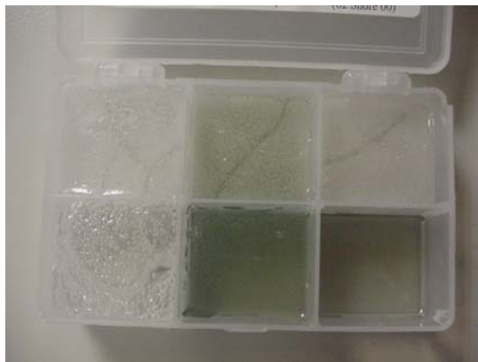
Figure 8 - Picture of silicone gels cooled below T_f and re-warmed to room temperature (1 day after warming)
