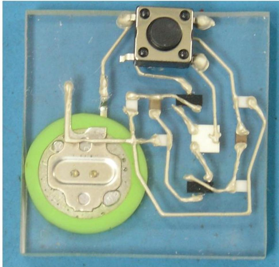
**Printing stretchable inks on elastomer bases potential**
