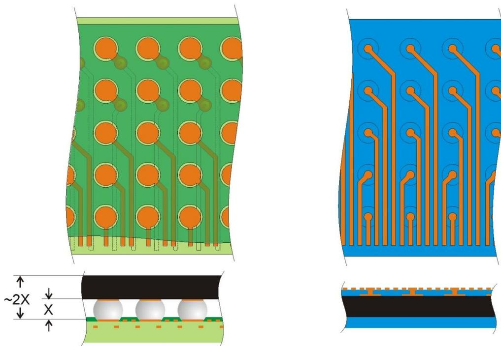
**Figure 4** at any given lead pitch, solderless assembly methods can significantly reduce both layer count by freeing up routing space and assembly height as solder often makes up half of the overall height of a mount package.
