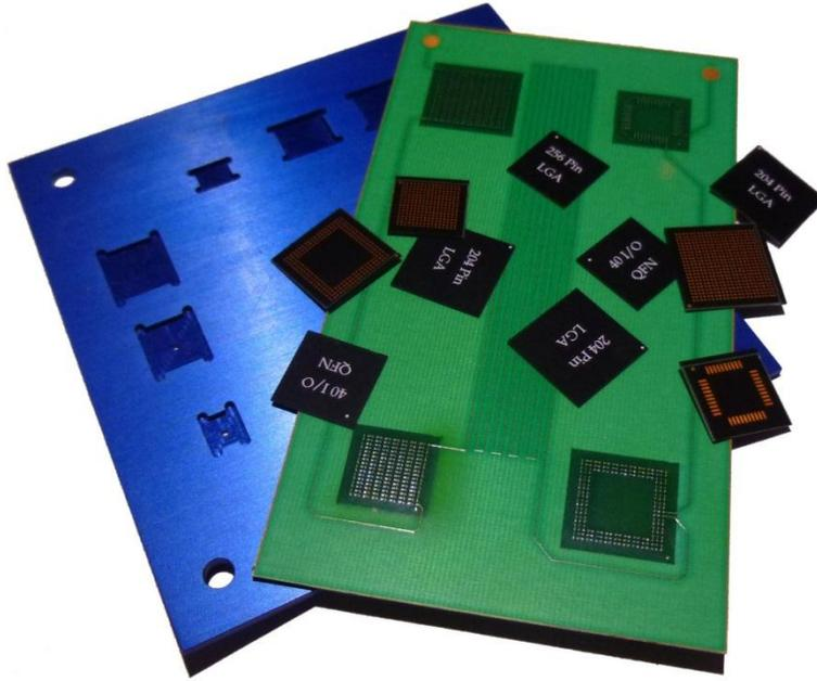
**Figure 1 Aluminum is a viable alternative to customarily used laminates when solder is not used to make interconnections between components and circuits. Aluminum is unique in that its surface can be anodized creating an insulation layer of alumina which can be colored and sealed. All components shown have a purposely selected 0.5mm contact pitch for reasons discussed in the text.**
