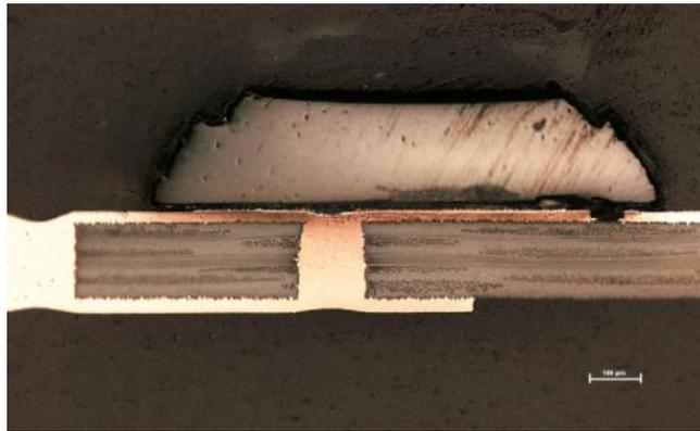
**Figure 18.** Chip carrier with dimple inside via
