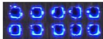
**Figure 11.** Images of bottom of stencil photographed under UV light after 10 prints with no under wipe
