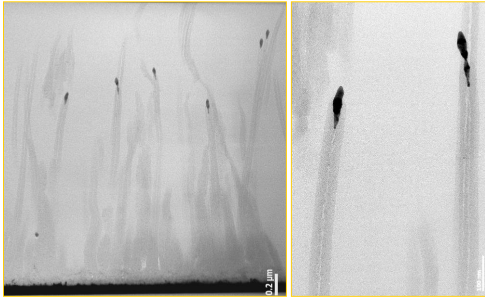
Fig. 2 Cross sectional view of CNFs rooted in a metal pad and wetted with solder. The dark area is the catalytic metal particle and the lighter area is the attached CNF.
