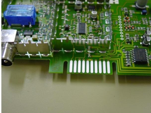
**Figure 1: Example of selective soldering metal shielding**
