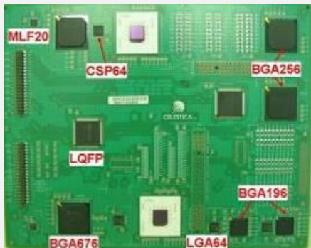
Celestica's RIA3 test vehicle used to evaluate manufacturing feasibility
