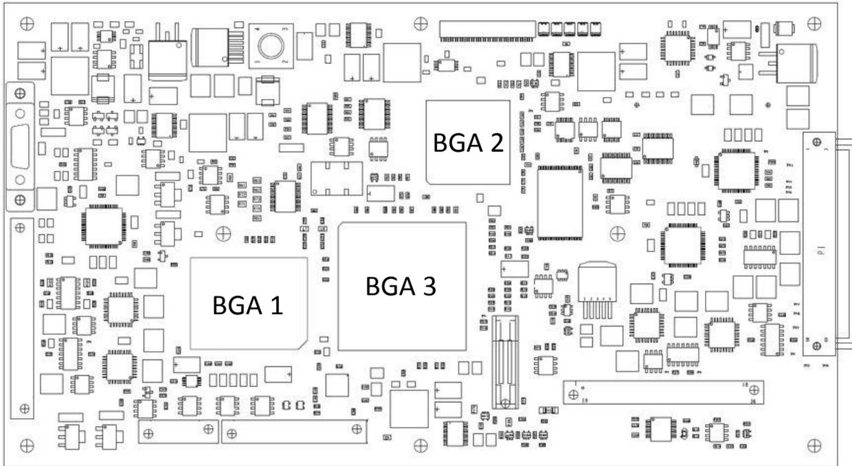
Figure 2 – Circuit card test vehicle top side layout
