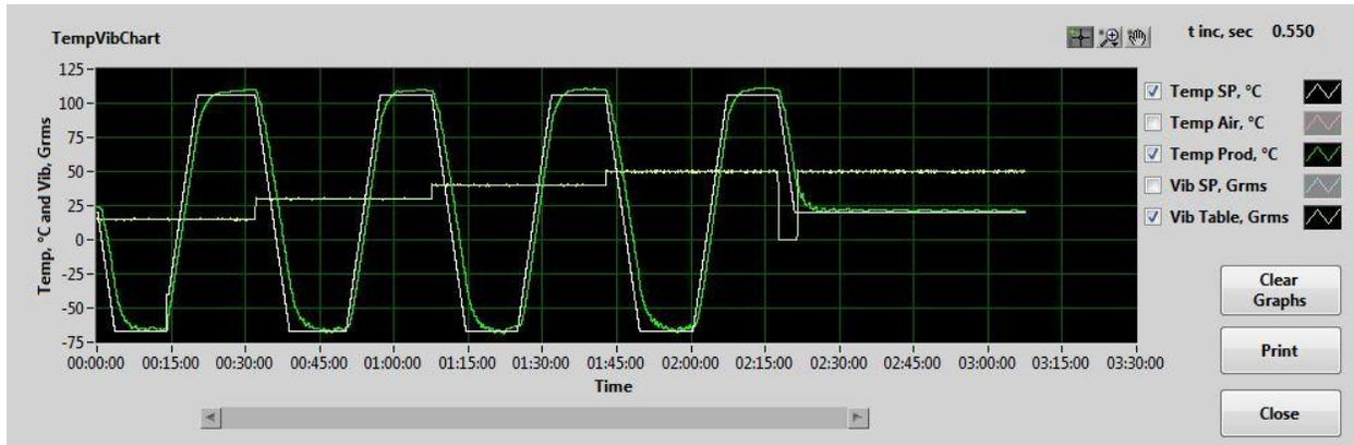
**Figure 7 – Combined thermal and vibratory profile for units in HALT, with extended vibe. The yellow line shows vibration input levels at the table, the grey line is the thermal program, and the green line is the thermal reading on one of the BGAs.**
