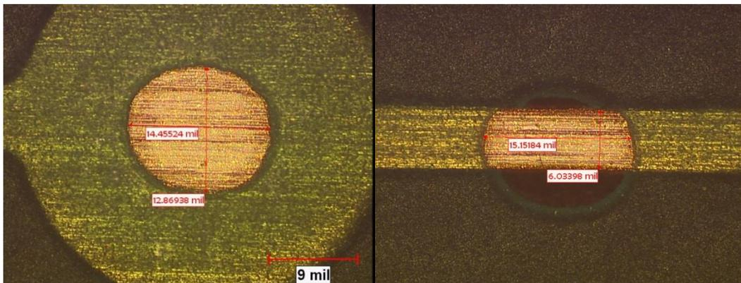
**Figure 3: Individual examples of Copper & SMO configurations**
