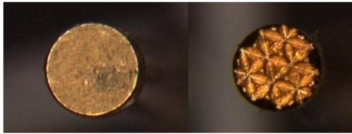
**Figure 4: Bead Probe Styles – Flat & Waffle**
