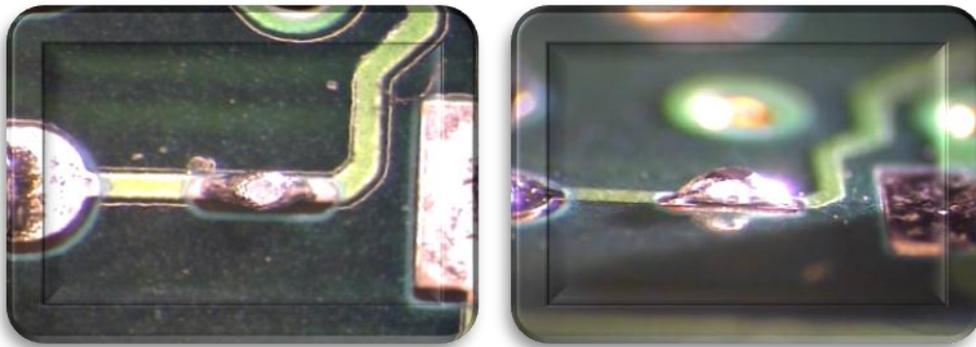
**Figure 8: Special Probing on small solder bump on trace**
