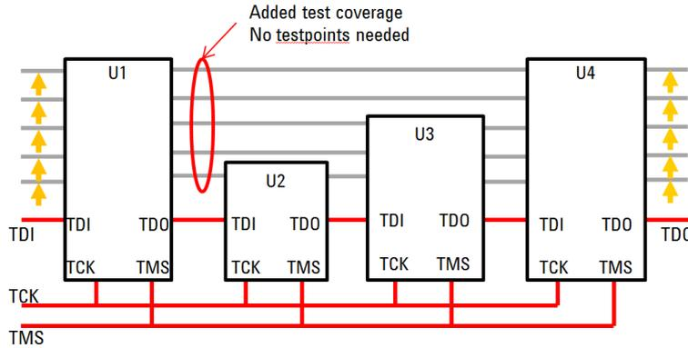
**Figure 3: Chain boundary scan devices to save on testpoints**
