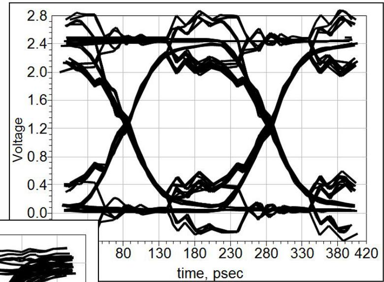
**Trace with 35 mil test target**
