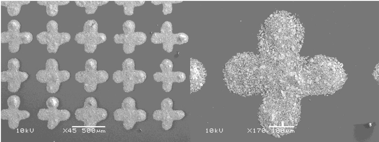
**Figure 7. SEM photos of printed silver epoxy patterns.**
