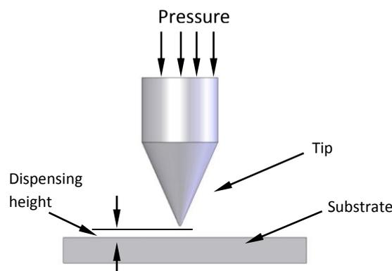
**Figure 2. Schematic drawing of the CFD model**
