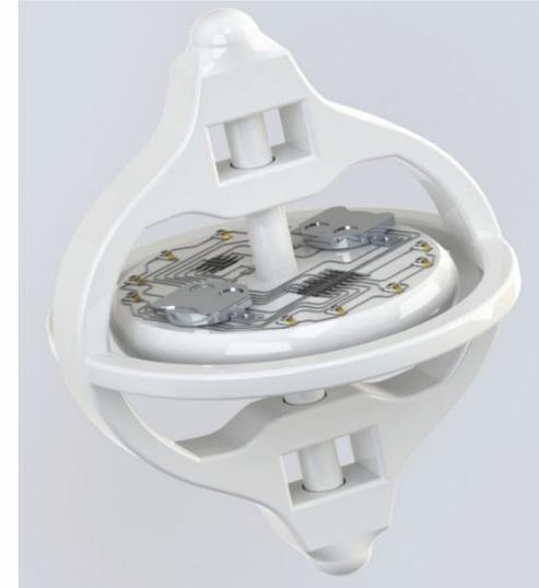
Structure is digitally printed with openings for the actives. Actives are placed upside down in the openings. Silver polymer is printed and including directly to the actives. Printed resistors are strategically placed and designed to accommodate the hole in the plastic.
