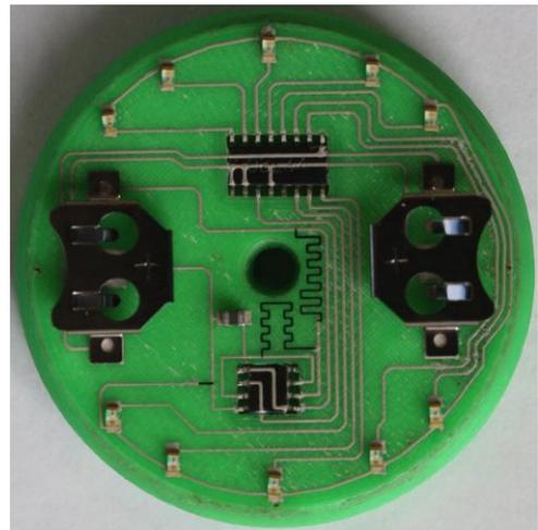
**Figure 11. 3D Printed Gyroscope Disc with components**
