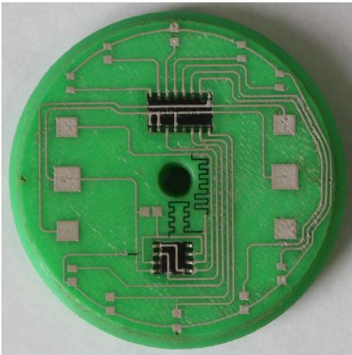
**Figure 10. 3D Printed Gyroscope Disc without components**
