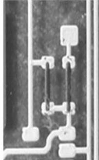
Printed strain gauges
