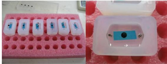
**Figure 18 – Fully Moulded Test Samples in Silicone Moulds**
