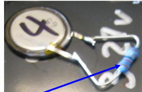
Load Resistor 18k $\Omega$
