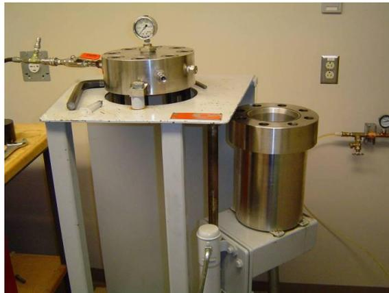
**Figure 19 – Hydraulic Pressure Vessel**
