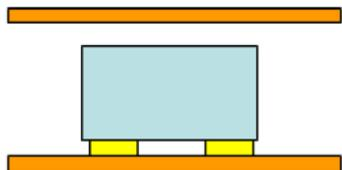
Component connected with pads and placed on side A
