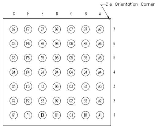
Figure 2 – Daisy chain test pattern on ITE2000EC
