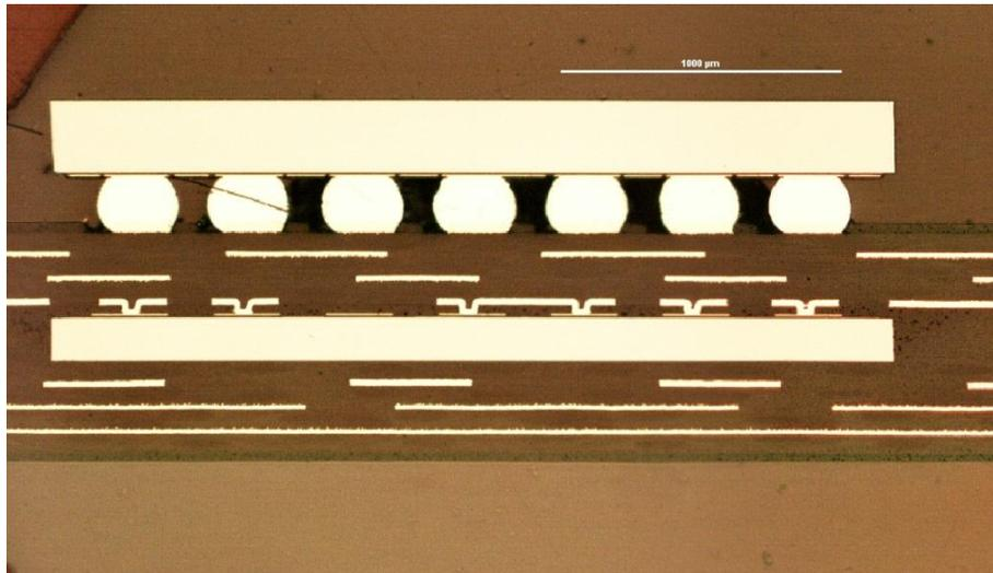
**Figure 6 - EC and SMD vary in z-axis dimension**
