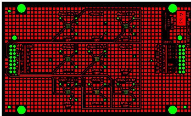
Figure 3 – Outer layer circuit pattern of ITE2000EC
