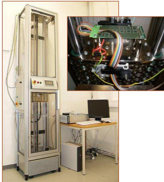
**Figure 8 – Drop Test Device and Test Terminal Set-up**
