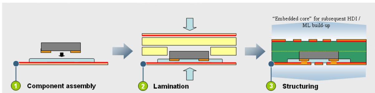
**Figure 7 – Basic assembly method of the embedded core**
