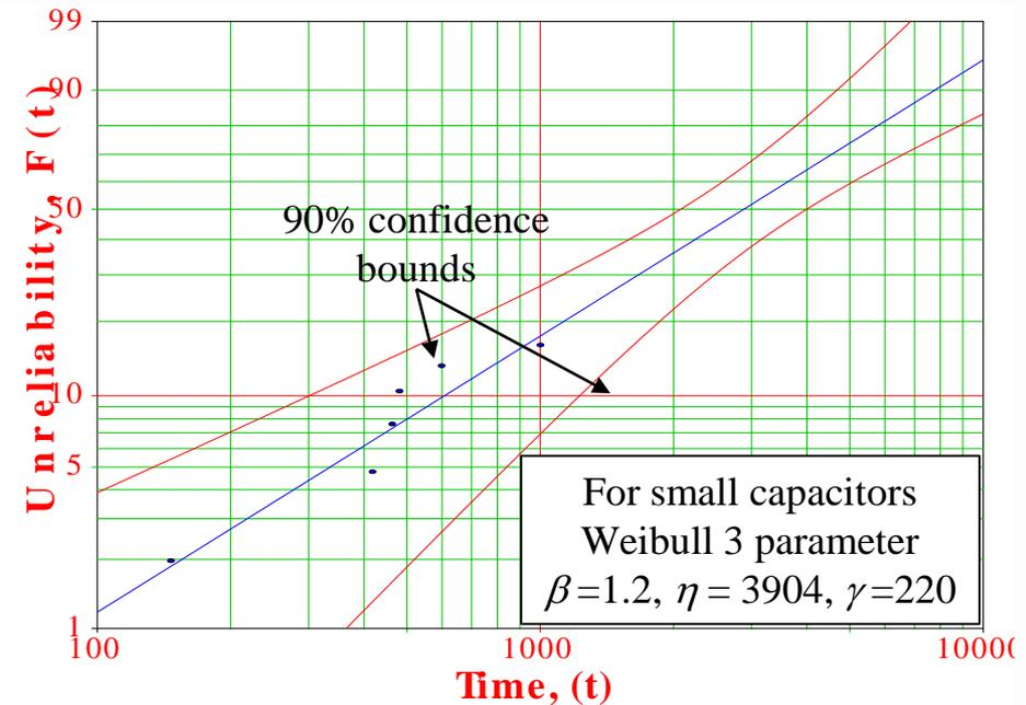
All failures as a result of formation of a conduction path disappeared after baking at 125°C for several days.
