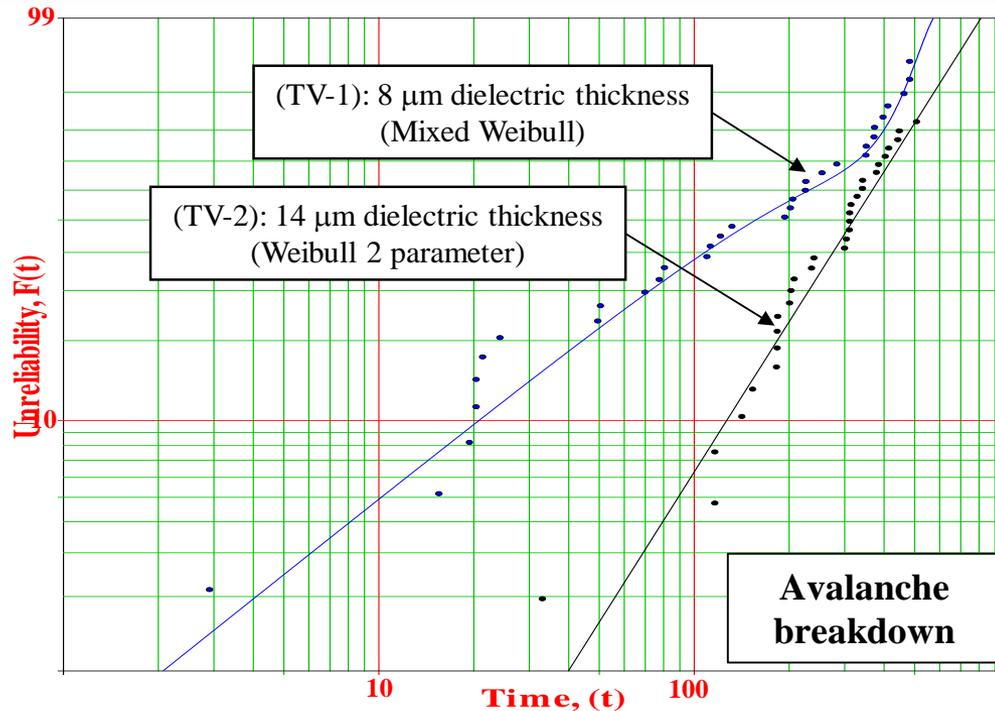
Type I failures were not observed in TV-2 (14  $\mu\text{m}$ )
