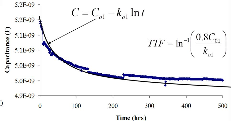
Failures were not observed in group B (large) capacitors due to a large value of initial capacitance ( $C_{o1}$ ) as compared to group A.
