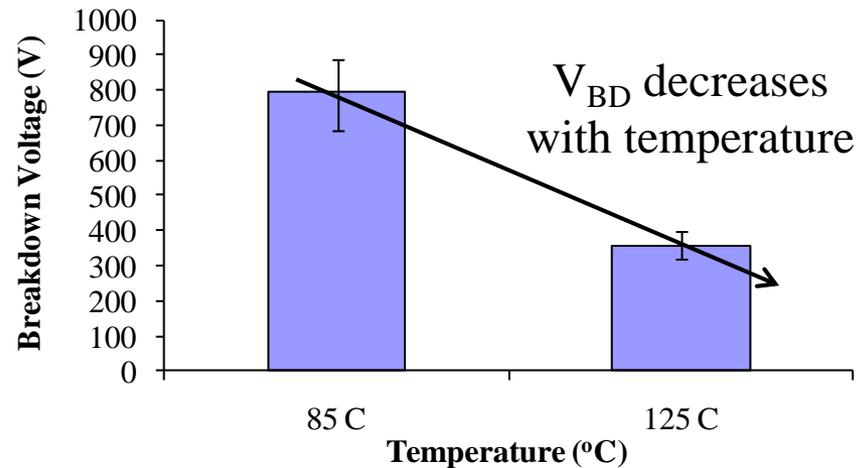
Measurement of breakdown voltage ( $V_{\text{BD}}$ ) on 10 small capacitors
