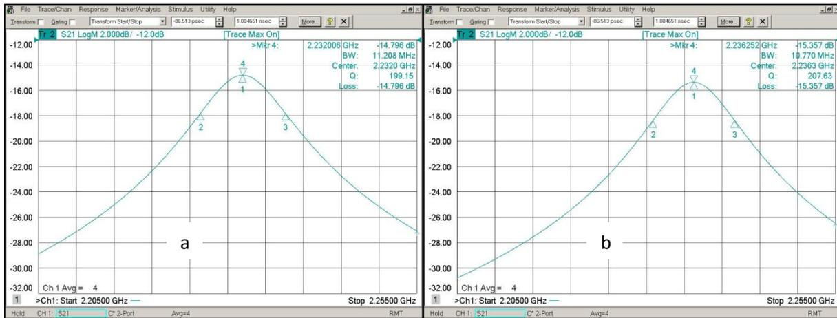
**Figure 4. Two screen-shots of the same microstrip gap coupled resonator using a substrate with a Dk of 12.2 (a) initial measurement and (b) is the measurement after the circuit is tested within a grounded enclosure.**
