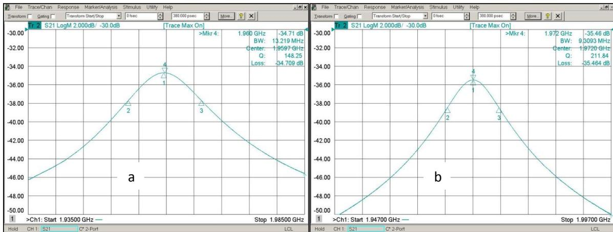
**Figure 3. Two screen-shots of the same microstrip gap coupled resonator using a substrate with a Dk of 4.5 (a) initial measurement and (b) is the measurement after the circuit is tested within a grounded enclosure.**
