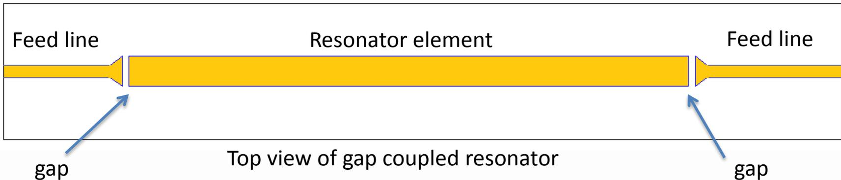
The resonator was designed on 30mil thick TMM<sup>®</sup>4 laminate (Dk=4.5), using  $\frac{1}{2}$  wavelength resonator at 1 GHz. The node that was tested was node 2 at approximately 2 GHz.
