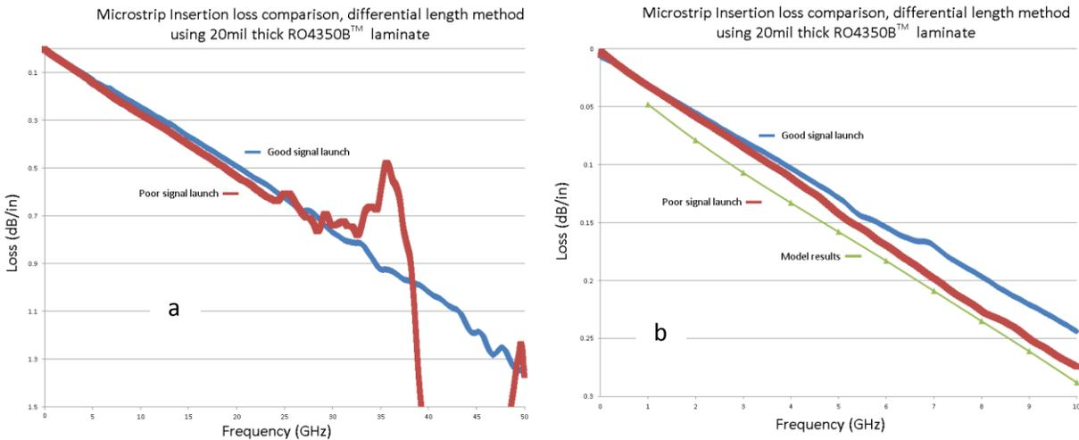
**Figure 7. Two sets of circuits were made from the same sheet of copper clad laminate, with the only difference being the signal launch design. Insertion loss curves shown with both sets across a (a) wide range of frequencies and (b) a lower range of frequencies.**
