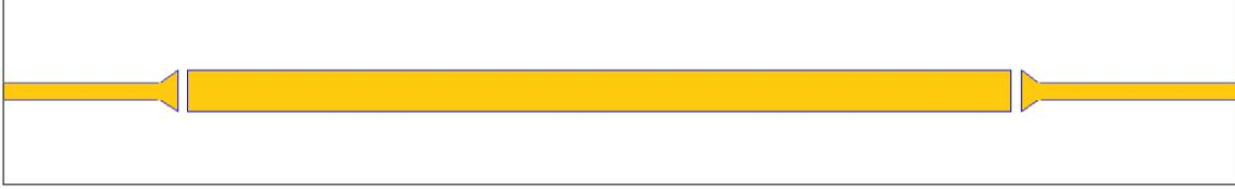
**Figure 2. Top view of a microstrip gap coupled resonator.**
