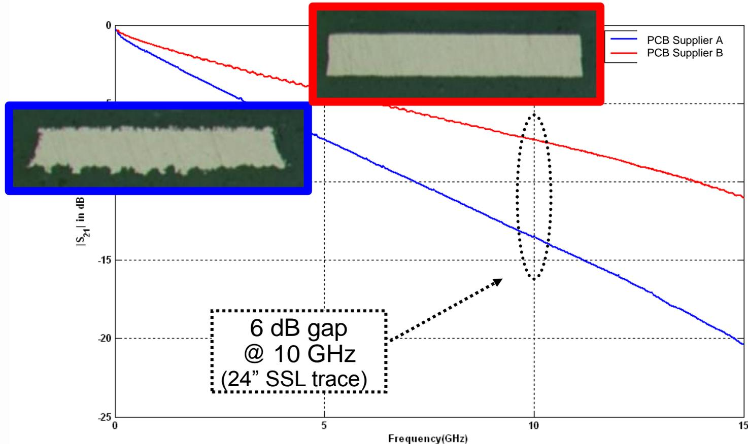
$|S_{21}|$  insertion loss of an SI test card built by two PCB suppliers, one with **rough** traces and one with **smooth**.
