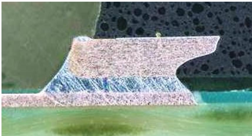
Figure 5 - QFN68 with 2.8 mil standoff height (Site B13)
