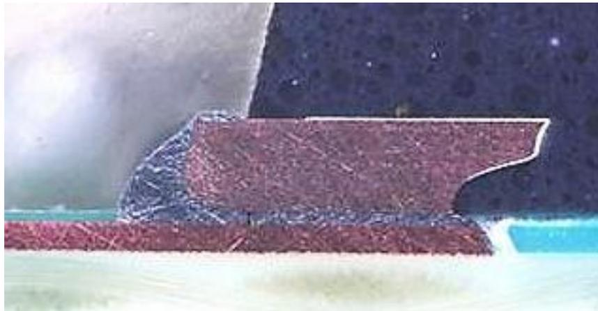
Figure 4 – QFN68 with 1.0 mil standoff height (Site B2)
