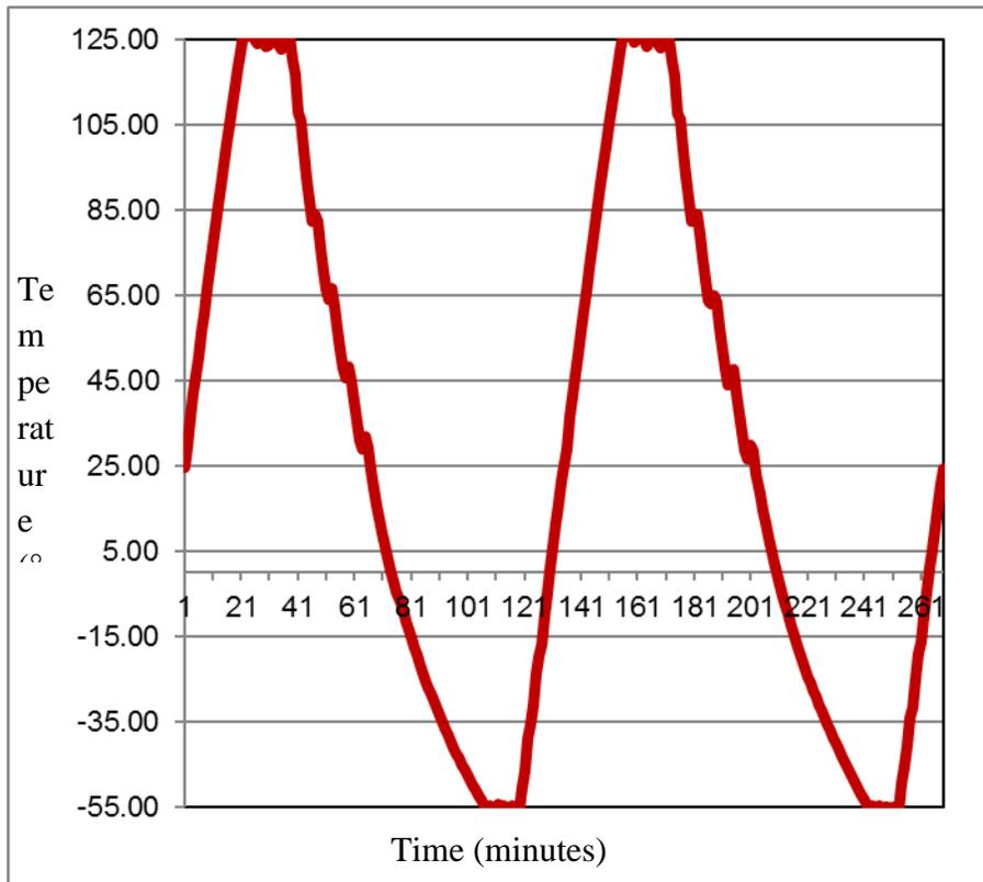
Figure 7 – Thermal cycle profile of test vehicles
