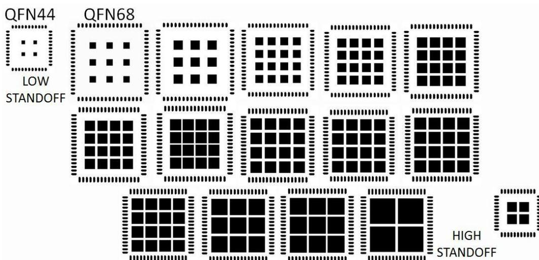
Figure 3 – Representative solder paste stencil apertures
