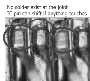
Figure 10 - Another Example of Poor Solder
