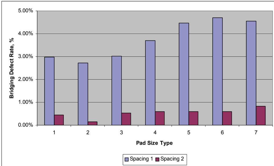
**Figure 19 - Bridging Defect Rate Comparison for Different Pad Size Types.**
