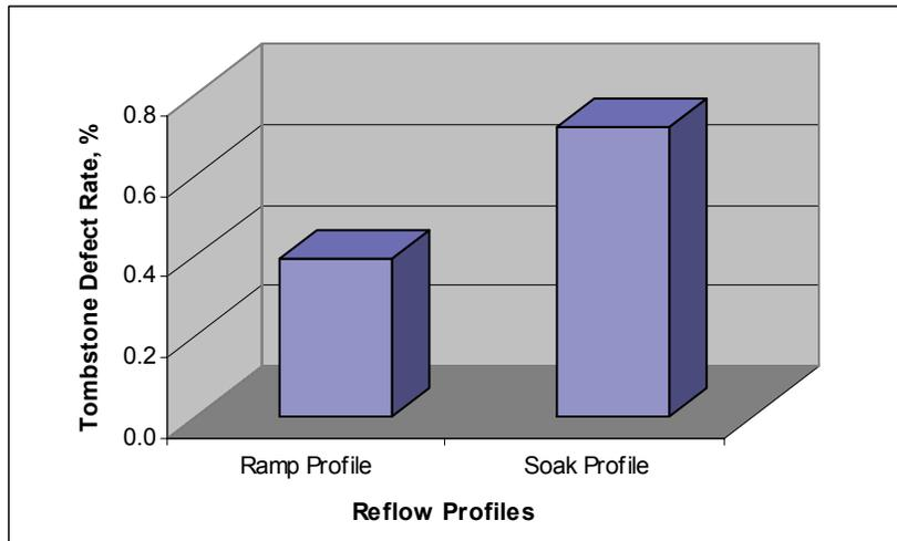
**Figure 21 - Tombstone Defect Rate as a Function of Reflow Profile.**
