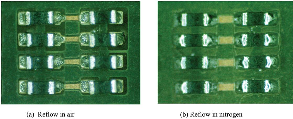
**Figure 15 - Wetting Comparison in Air (a) or Nitrogen (b).**
