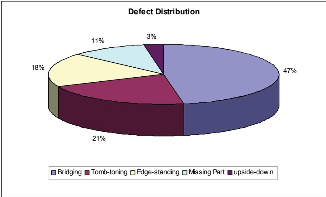
Figure 17 - Defect Distribution for all Build Combinations.
