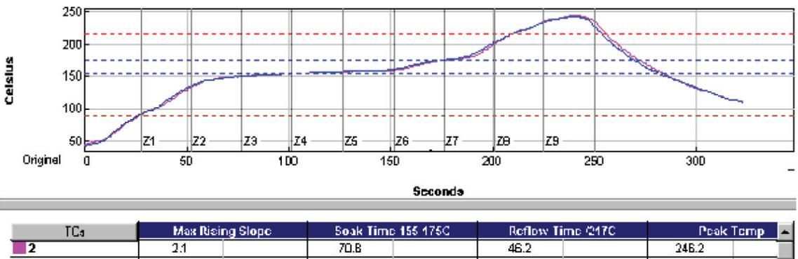
Figure 14 - Lead Free Soak Reflow Profile.
