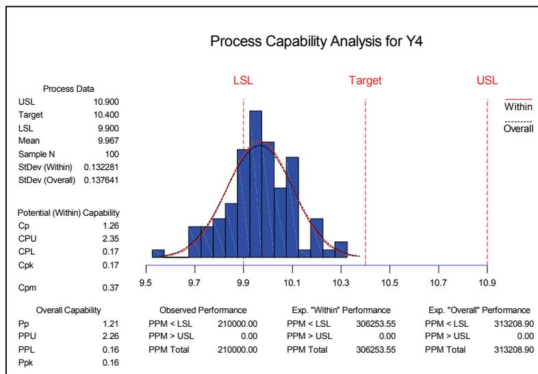
**Figure 2 - Capability Histogram for Y4 (Pad Size 4).**
