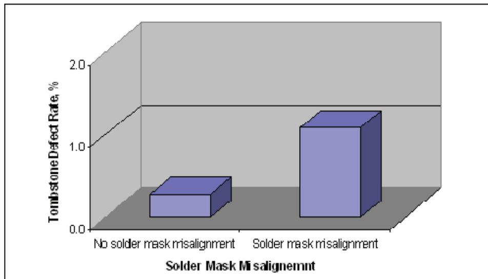
**Figure 24 - Tombstone Defect Rate as a Function of Solder Mask Misalignment for Pad Size Type 1.**
