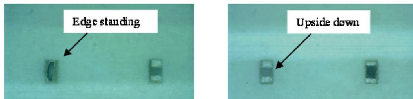
Figure 11 - Two Common Orientation Defects in As-received 01005 Components in Carrier Tape.
