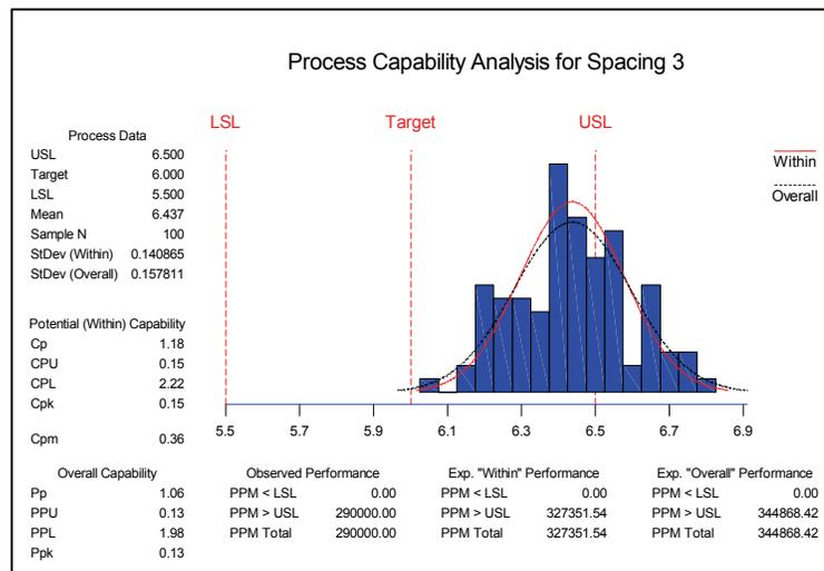
**Figure 3 - Capability Histogram for Pad-to-Pad Spacing 3.**
