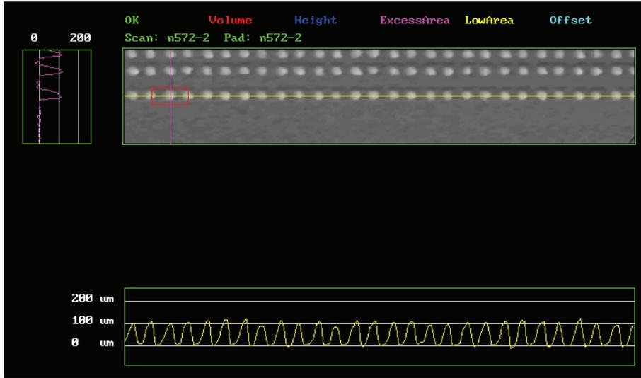
**Figure 5 - 3D Solder Paste Inspection Using the MVT SP-1 after Calibration.**
