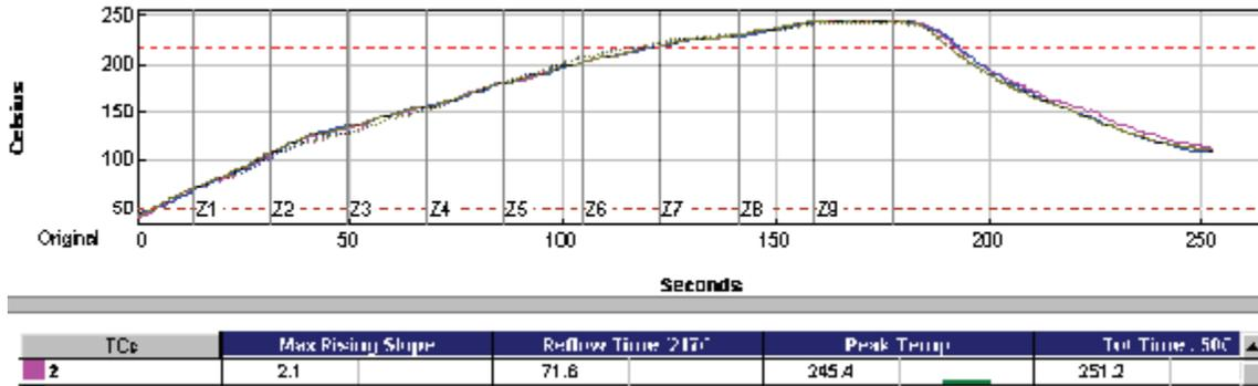
Figure 13 - Lead Free Quick-ramp Reflow Profile.
