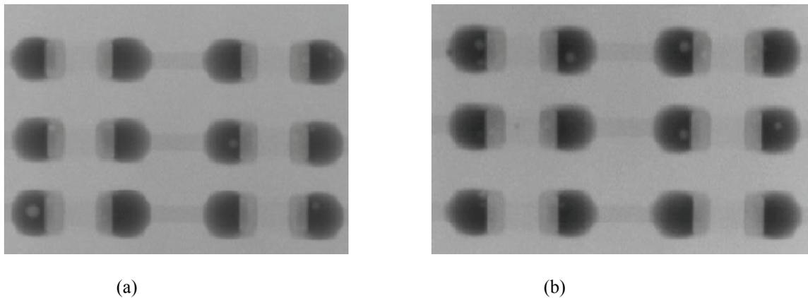
**Figure 16 - X-ray of Solder Joints for Ramp (a) and Soak (b) Profiles in Nitrogen.**
