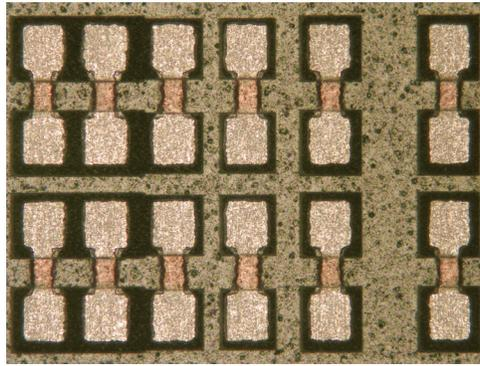
**Figure 4 - Photograph of Pads and Solder Mask Showing Lack of Solder Mask between Pads with 4 mil and 5mil spacing. The other pad spacings are 6mils, 8mils and 15mils.**
