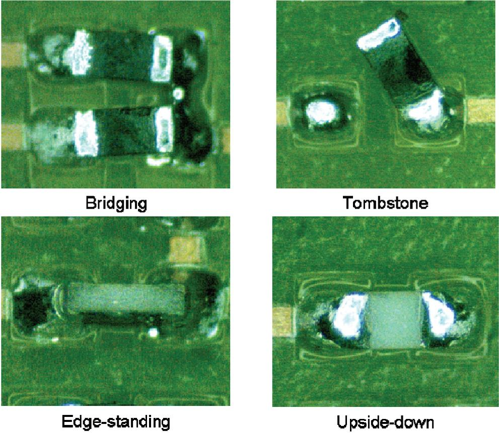
Figure 18 - Example of Different Defects.
