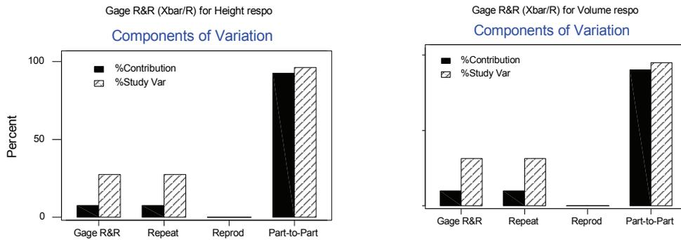
**Figure 6 - Gage R&R for Height and Volume Response.**
