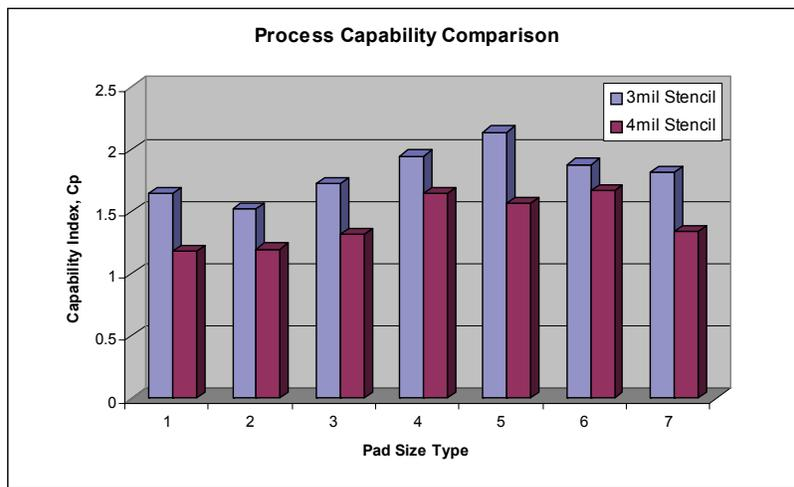
Figure 10 - Process Capability Comparison for Two Stencils and Different Pad Size Types.
