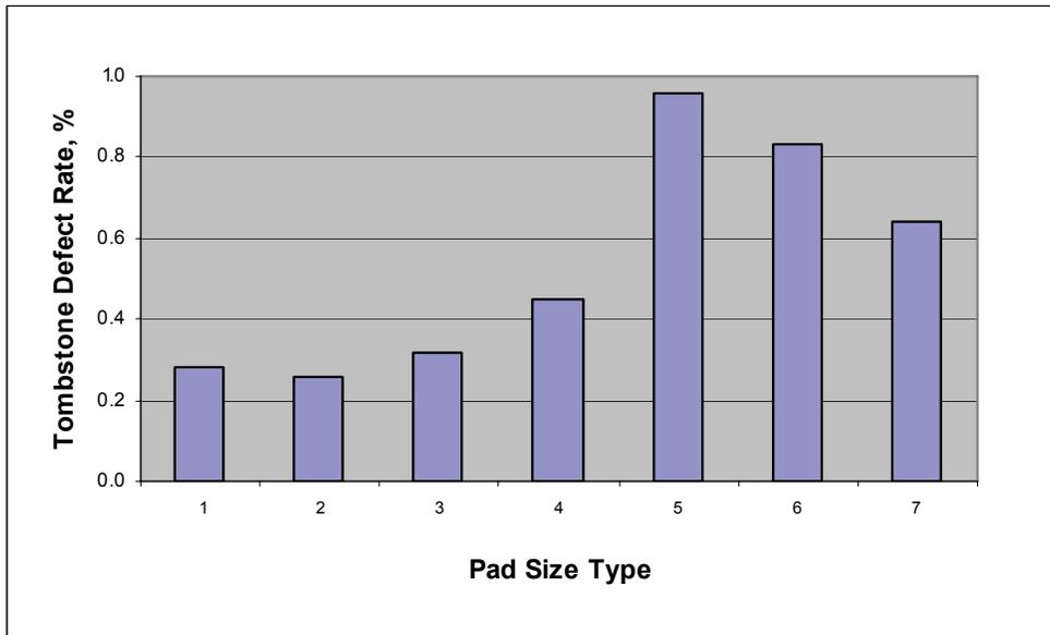
**Figure 23 - Tombstone Defect Rate as a Function of Pad Size Type.**
