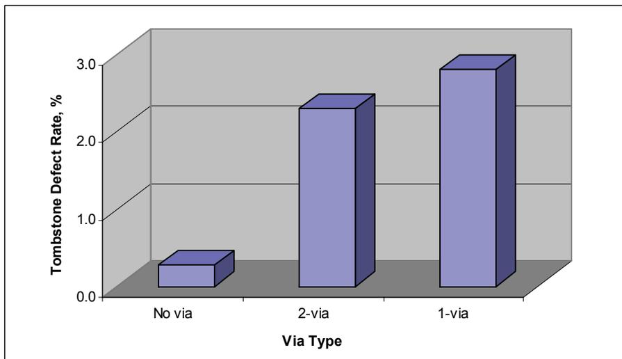
**Figure 20 - Tombstone Defect Rate Comparison for Pad Size Type 1 with and without Vias-in-Pad.**
