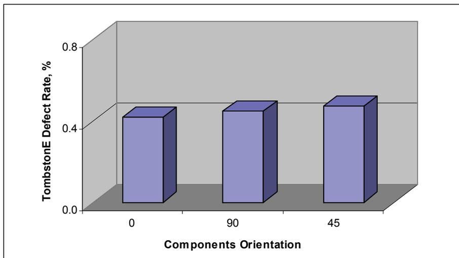
**Figure 22 - Tombstone Defect Rate as a Function of Resistor Orientation for Type 1 Size Pads.**
