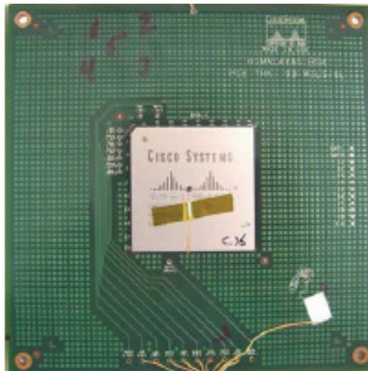
**Figure 4 - Test board Assembled with 45mm FCBGA for Reliability Testing**
