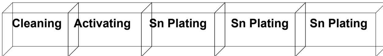
**Figure 8 - Production line set up for traditional leadframe plating**
