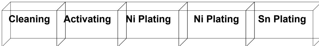
**Figure 9 - Plating line set up for thin Sn over Ni technology**
