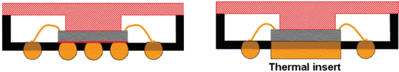
Figure 13 – Heat Management Package Designs
