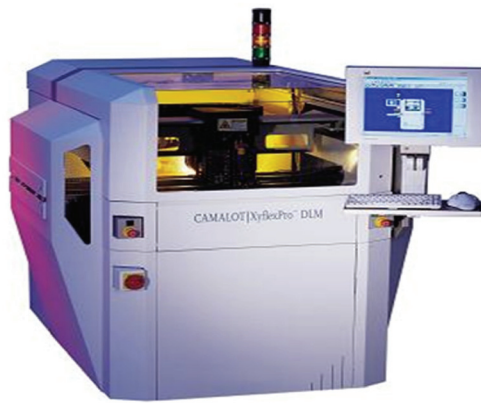
Figure 3 – XyflexPro Dual Line Dispenser
