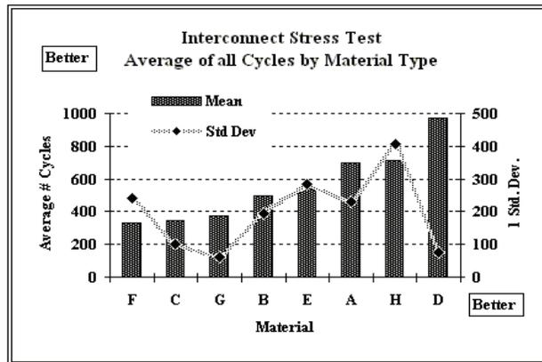
Figure 12 - IST Mean Cycles & S.D. for All Conditions by Material
