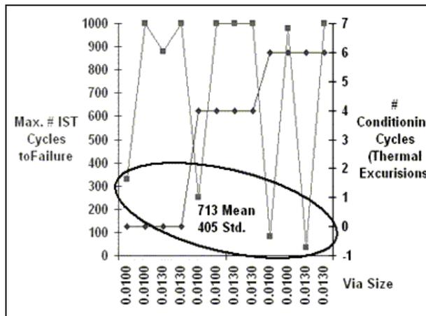
Figure 13 - Material “H” Showing Bimodal Response, not Reflow Dependent
