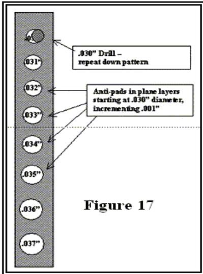
Figure 17 - A Depiction of the PTH-Wall-to-Copper Plane CAF Coupon
