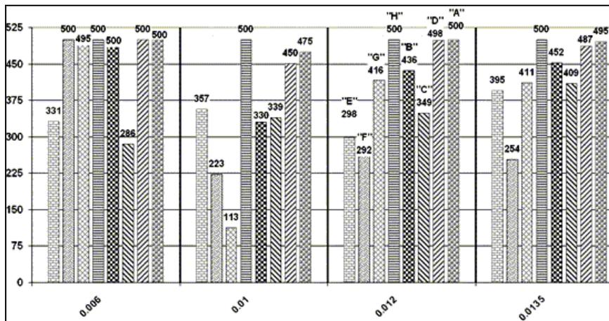
Figure 11 – Average of HATS Cycles for Each Material by Via Size for all Preconditions
