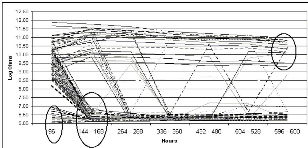
**Figure 25 – Material with a Large Number of Excluded (Circled at 96 hours), a Large Number of Early Fails (Circled at 144-168 hours), and Then Some Fails as Time Progressed**
