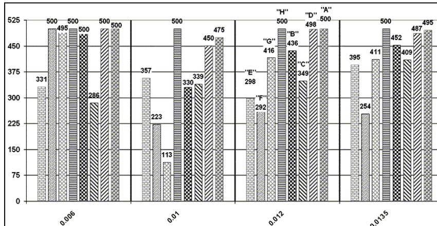
Figure 10 – Average of HATS Cycles for Each Material by Preconditioning for all Vias
