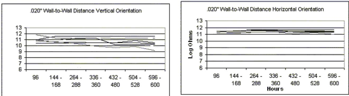
Figure 23 – Both Vertical and Horizontal Nets Passed Down to 0.51 mm [.020"] Spacing
