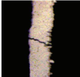
**Figure 2 - Copper Along a Hole Wall which was Cracked by Repeated High Material Expansion and Contraction**
