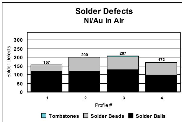
Figure 5 - Reflow Related Defects
