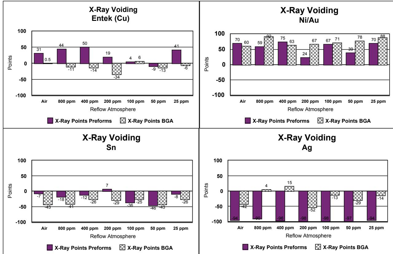
Figure 9 - Board Finish/Atmosphere Effects on Voiding
