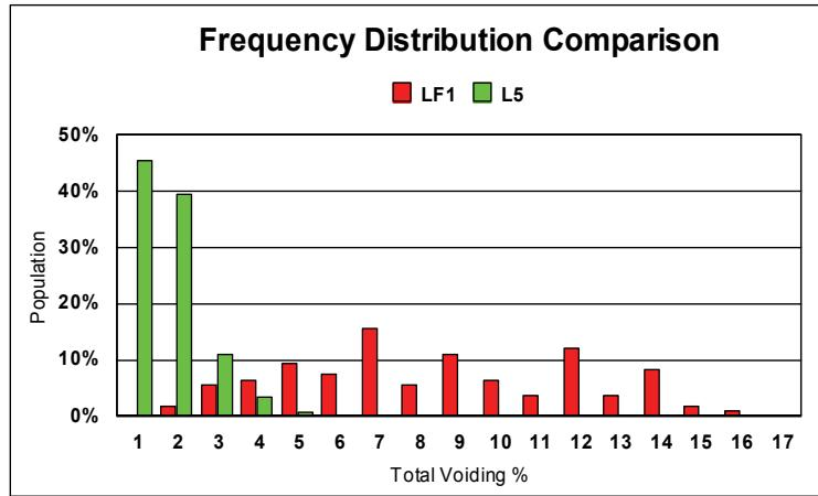
**Figure 3 - Sn/Ag/Cu Vs Sn/Pb**
