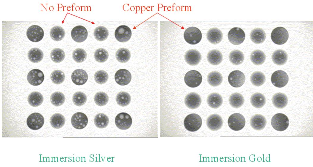
Figure 10 - Severe Voiding over Immersion Silver in 25ppm O<sub>2</sub>
