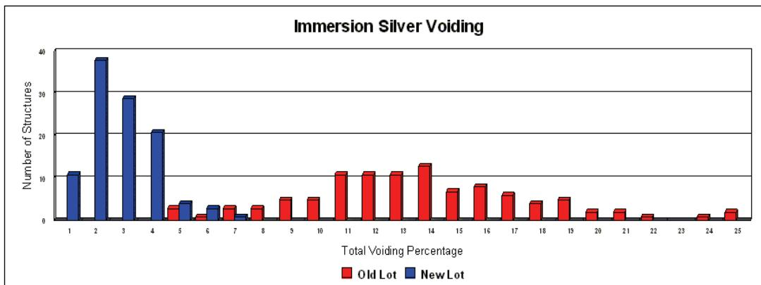
**Figure 16 - Voids Caused by Ag Finish Thickness**
