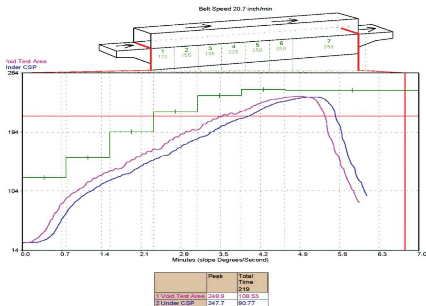
Figure 8 - Profile 2 with Longer Liquidus Time
