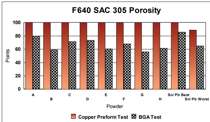
Figure 11 - Comparative Voiding Performance for 3% Ag SAC Alloy
