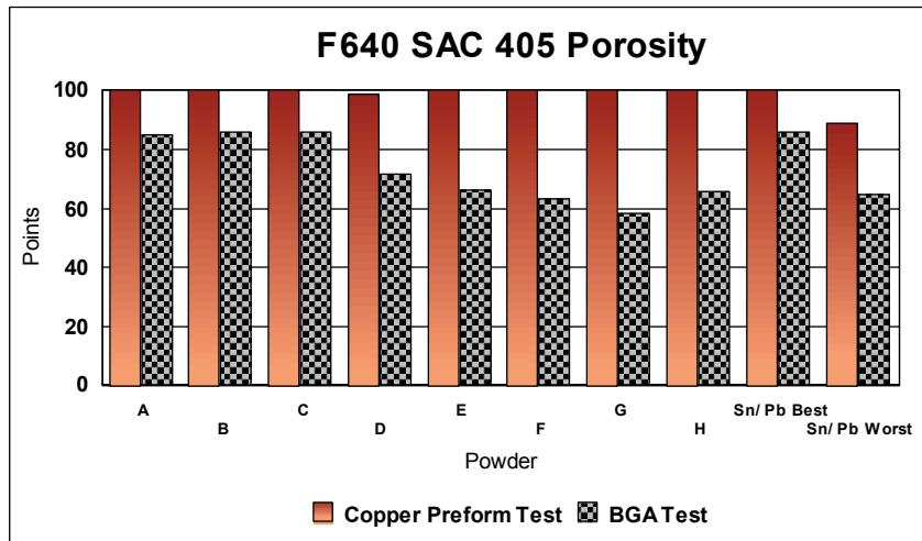
Figure 12 - Comparative Voiding Performance for 4% Ag SAC Alloy
