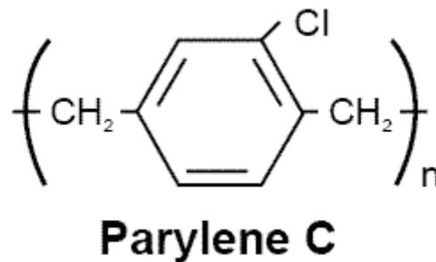
Figure 4 - Parylene C Molecular Structure
