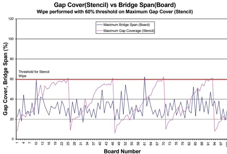
**Figure 3 - Maximum Gap Cover on Stencil (pink) and Maximum Bridge Span on Board (dark blue). Stencil wipe triggered when paste between aperture of the stencil reaches 60%**
