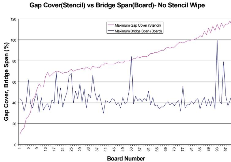
**Figure 2 - Maximum Gap Cover on the Stencil (pink) and Maximum Bridge Span on Board (dark blue). No stencil wipe**
