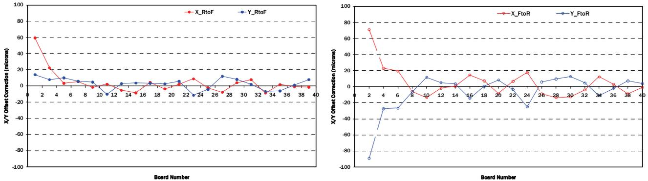
**Figure 1 - X and Y Print Offset Correction Results for RtoF stroke (Left) and for FtoR Stroke (Right)**
