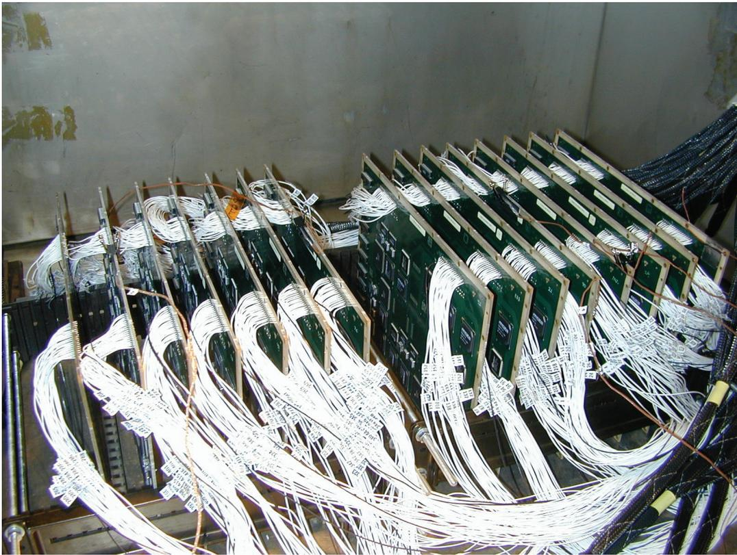
Figure 3 – Test Vehicles in Thermal Cycle Chamber
