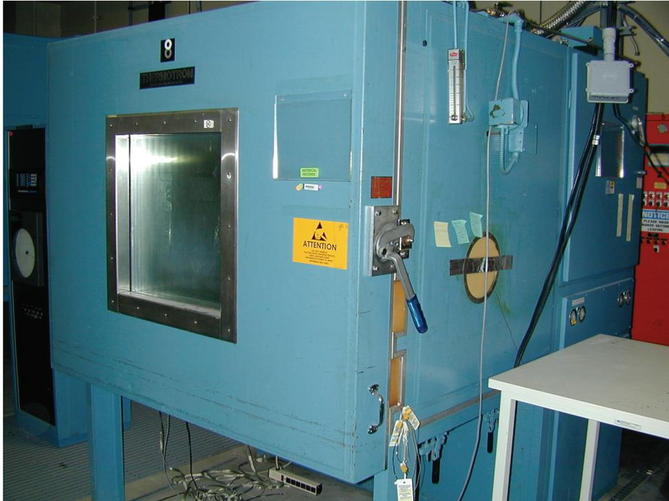
**Figure 2 - Thermal Cycle Chamber**
