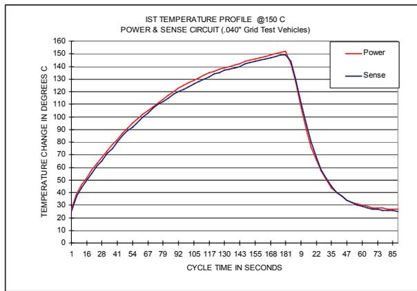
**Figure 2 - IST Cycle Temperature Profile**
