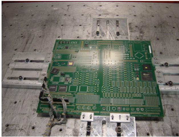
**Figure 8 – PWB in HALT Chamber**
