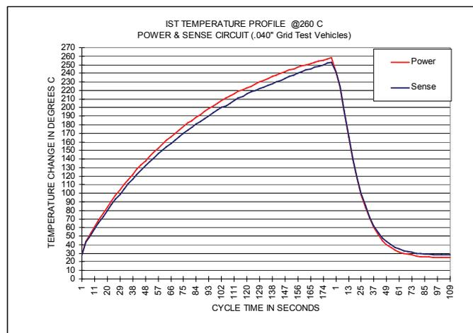
**Figure 1 - IST Preconditioning Temperature Profile**
