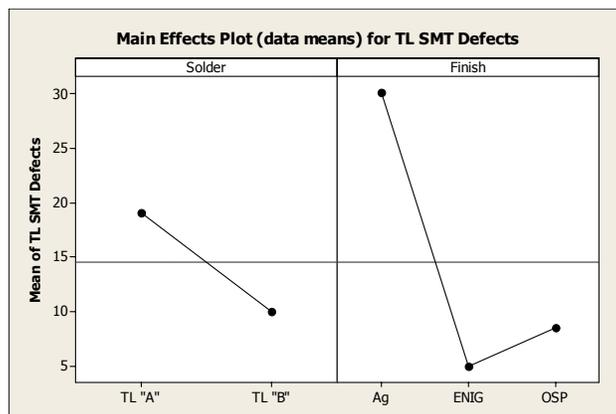
**Figure 5 - Mean SMT Defects per Tin/Lead PWB**
