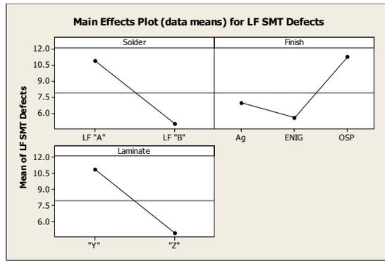
**Figure 3 - Mean SMT Defects Per Lead-free PWB**
