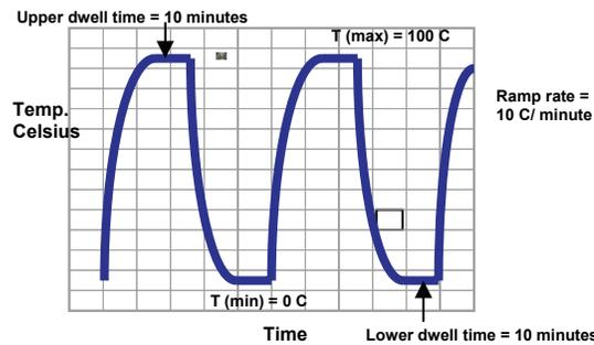
**Figure 6 – Thermal Cycling Profile**
