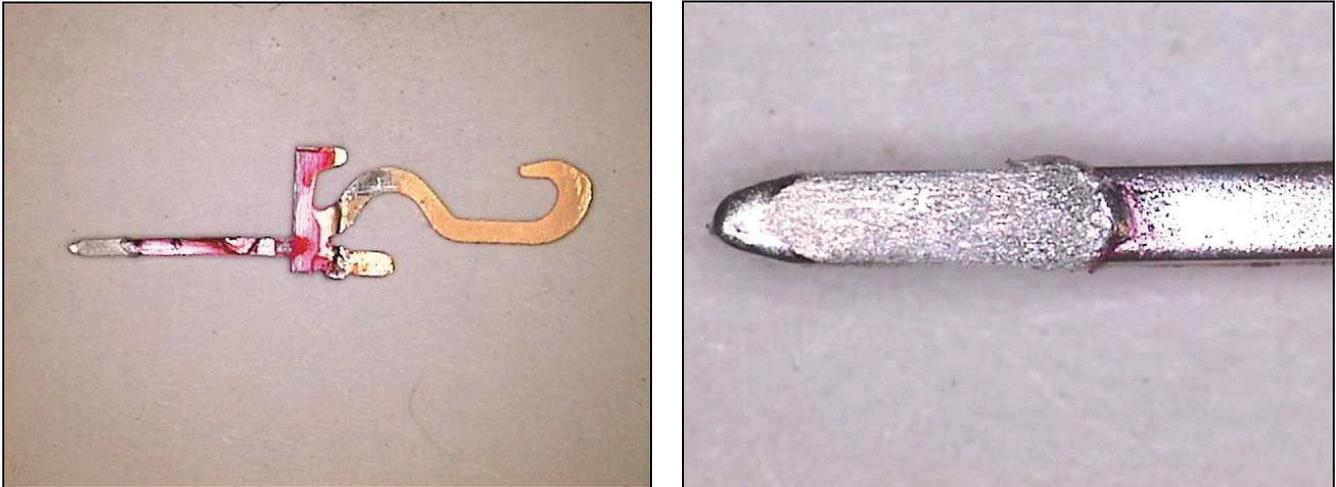
**Figure 3: Pin extracted showing solder wetting mark**
