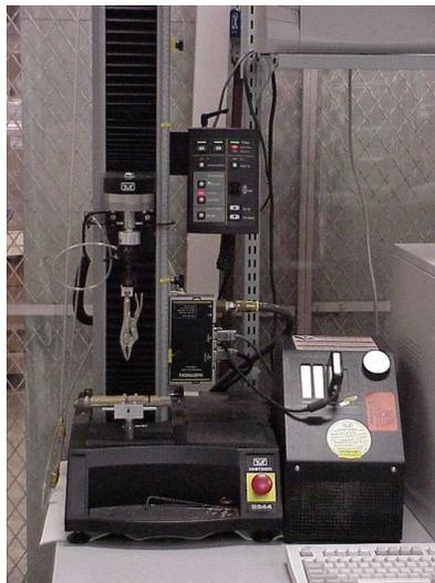
**Figure 2: Tester with modified vise grip and fixture**
