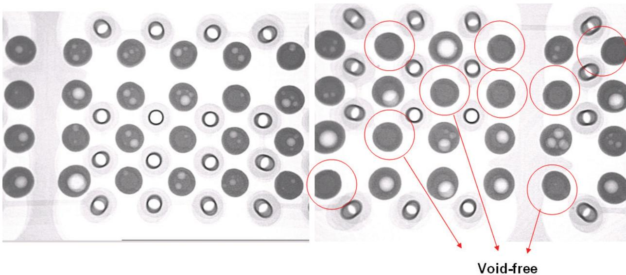
**Figure 5 - X-ray Pictures of Voids Distributed in Eutectic Solder Joints in 144 I/O BGA Reflowed Using Extreme Profile**
