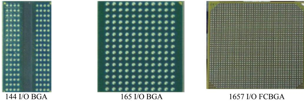
Figure 1 - Solder Ball Arrays in Three BGA Packages
