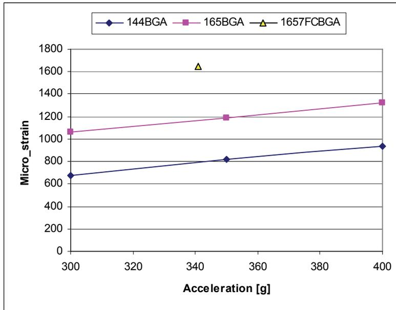
Figure 7 - Max. Principle Strain Measured During Shock Test
