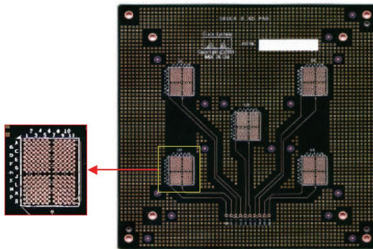
Figure 2 – Test Vehicle for 165 I/O BGA
