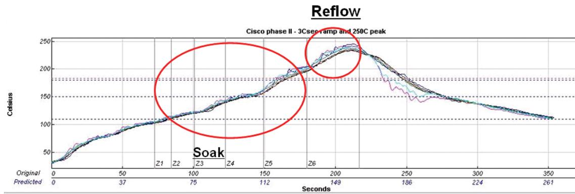
Figure 8 - Extreme Reflow Profile with 3C/sec ramp and 250C Peak
