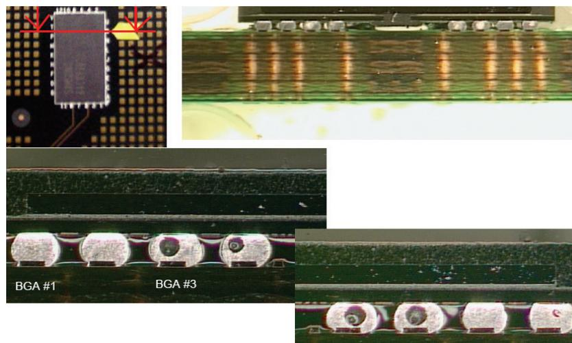
**Figure 12 - Void Distribution in 2%Ag Solder Joints in Preconditioned 144 I/O BGA Assembled with the Extreme Profile**
