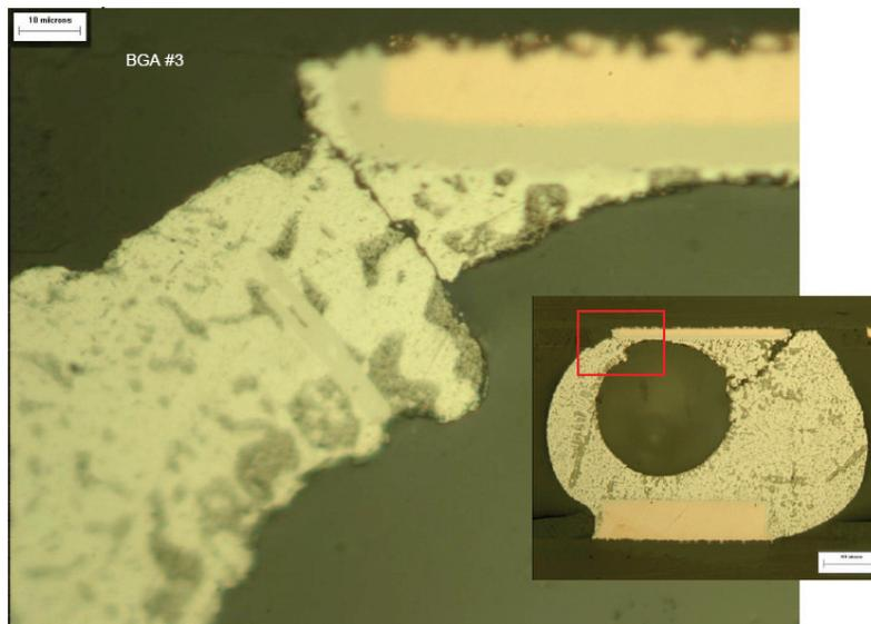
**Figure 11 - Crack Propagation in a Large Void-Containing 2%Ag Solder Joint in a 144 I/O BGA Assembled with the Extreme Profile**
