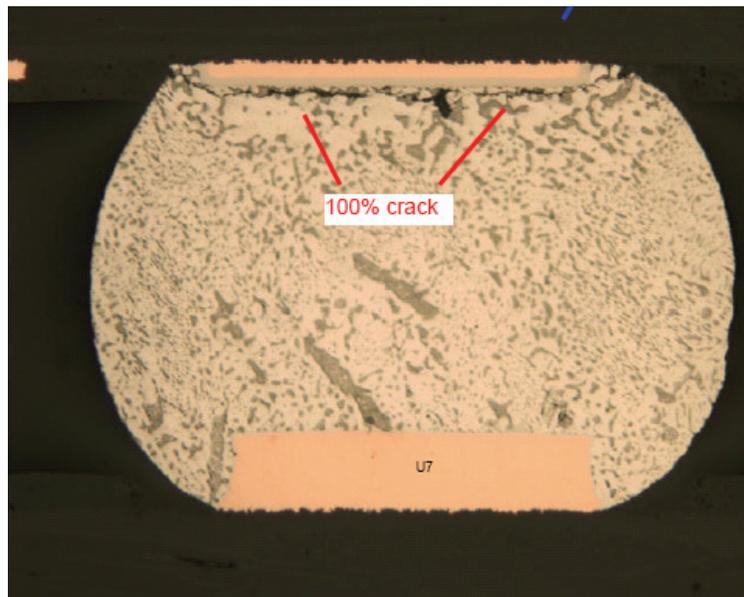
**Figure 10 - Crack Propagation in a Void-free 2%Ag Solder Joint in 144BGA Assembled at LSLP Profile**
