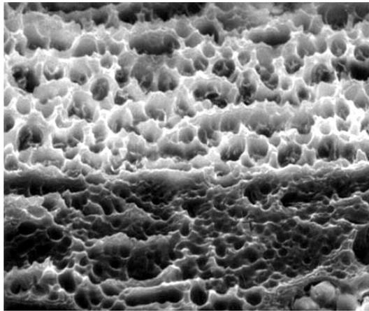
**Figure 2 - High Tg Material after Alkaline Permanganate Desmear.**
