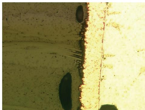
**Figure 4a - Resin Voiding from Solvent Retention.**
