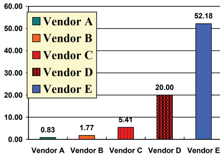
**Figure 9 - Y-Axis Denotes the Percentage of Interconnects that Display at the Least a Hairline Fracture after 6X Solder Floats.**
