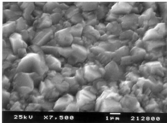
**Figure 12 - Tight Grained and Angular Deposit of Copper on the Interconnect.**
