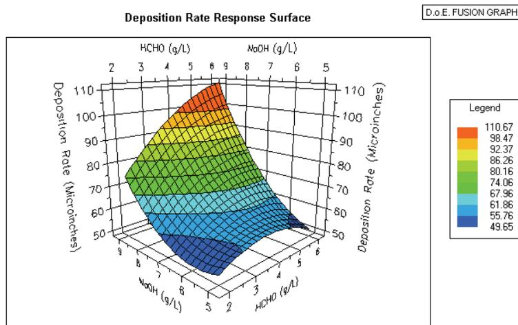
**Figure 10 - Deposition Rate of Electroless Copper as Influenced by Sodium Hydroxide Content and Formaldehyde Concentration.**
