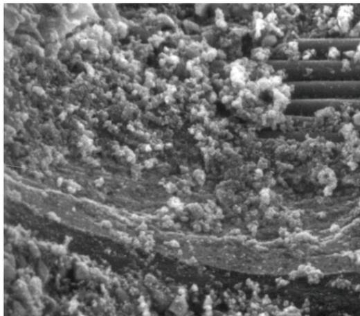
**Figure 1 - High Tg FR-4 Material After drill. Note Debris on Hole Wall from Drilling**
