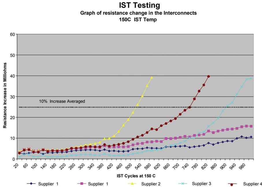
**Figure 6 - IST Results From Four Commercially Available Electroless Copper Processes.**
