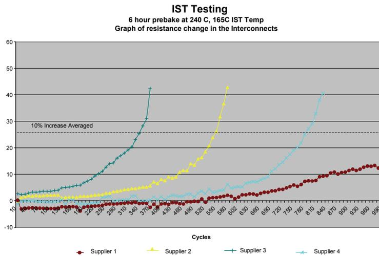
**Figure 7 - IST Results from Four Commercially Available Electroless Copper Processes. Results obtained after preconditioning the test coupons for six hours at 240 C.**
