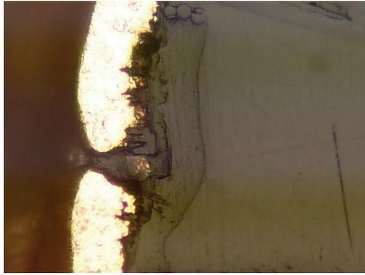
**Figure 4b - Example of Electroless Copper Voiding Due to Solvent Retention.**
