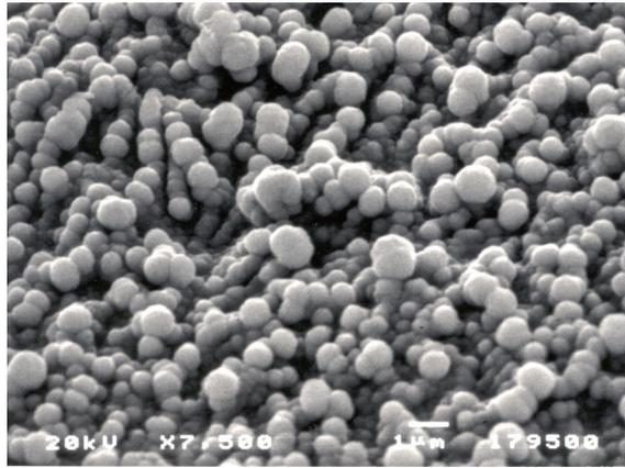
**Figure 13 - Large and Loose Grain of Electroless Copper Deposit from a Fast Deposition rate Electroless Copper Process.**
