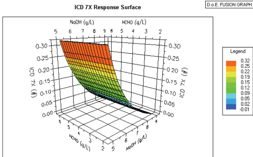
**Figure 11 - ICD Response Based on Interaction of Formaldehyde and Sodium Hydroxide Concentrations. ICD's Determined After 7 X solder Floats. ICD Test Vehicle as Described in Figure 7.**
