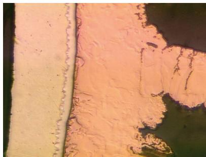
**Figure 5 - Microcracks Present after IST Cycling**
