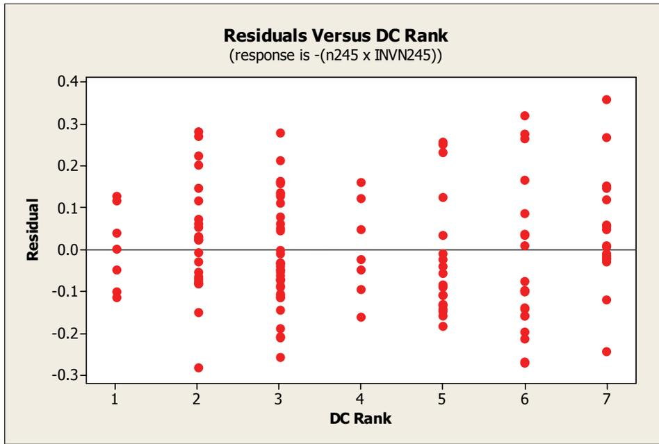
**Graph 9 – Standardized residual plot versus the DC (date code) rank. There does not seem to be a trend between date codes. Therefore, the final regression model does not include a term for the data code.**
