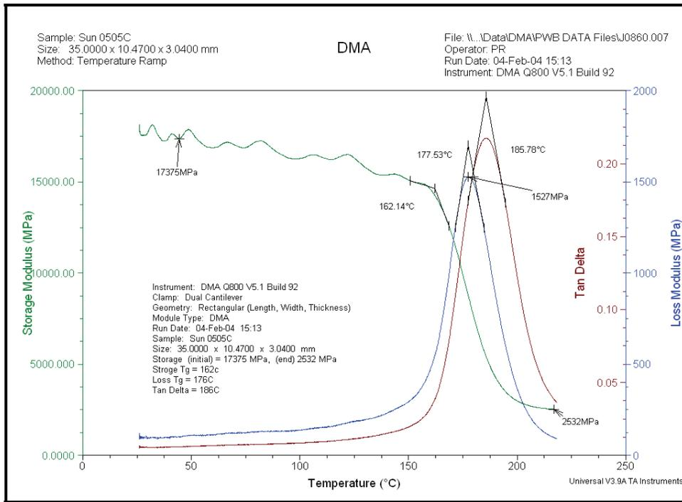
**Graph 12 – DMA plot of modulus versus temperature for board date code 0505C.**
