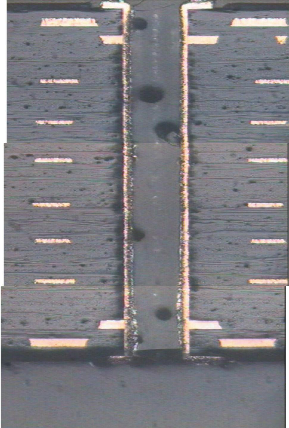
**Coupon # 0805C-5989B - Mean Cu = .0013" – 1691 Cycles – PTH Failure**
