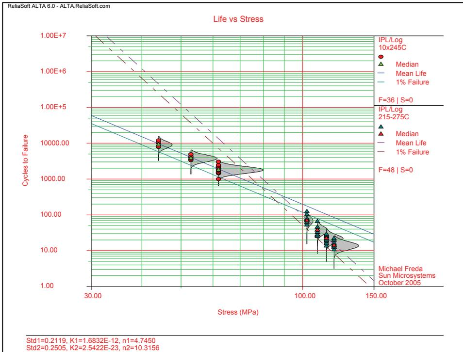
**Graph 16 – The plot uses IPL/Lognormal of stress versus cycles to failure. Separate estimates made below and above Tg due to preconditioning of 10x at 245°C below Tg.**
