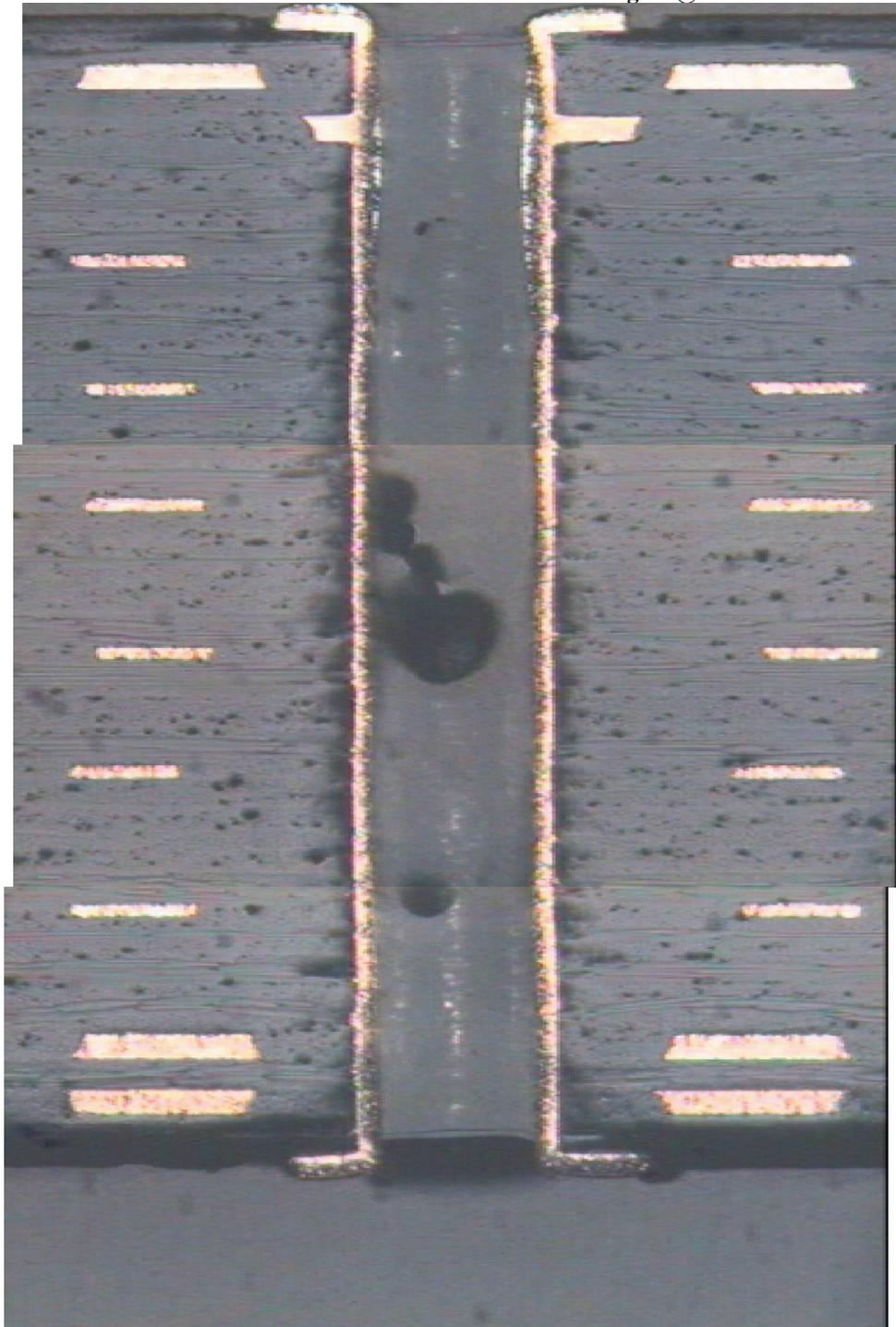
**Coupon # 0805E-5890A - Mean Cu = .0013" – 3877 Cycles – PTH Failure**
