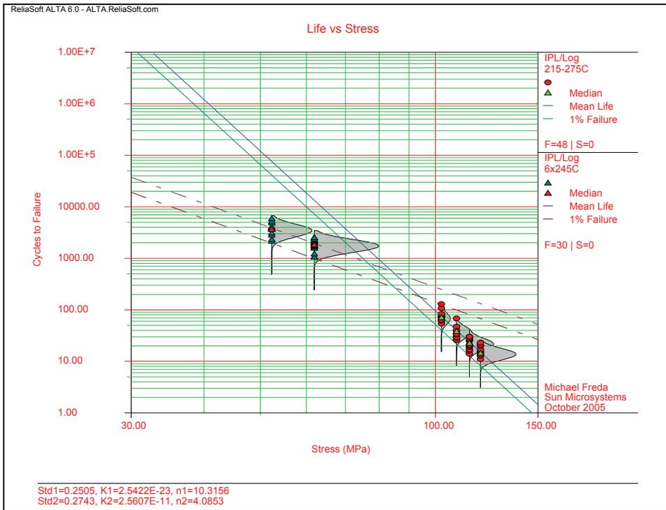
**Graph 15 – The plot uses IPL/Lognormal of stress versus cycles to failure. Separate estimates made below and above Tg due to preconditioning of 6x at 245°C below Tg.**
