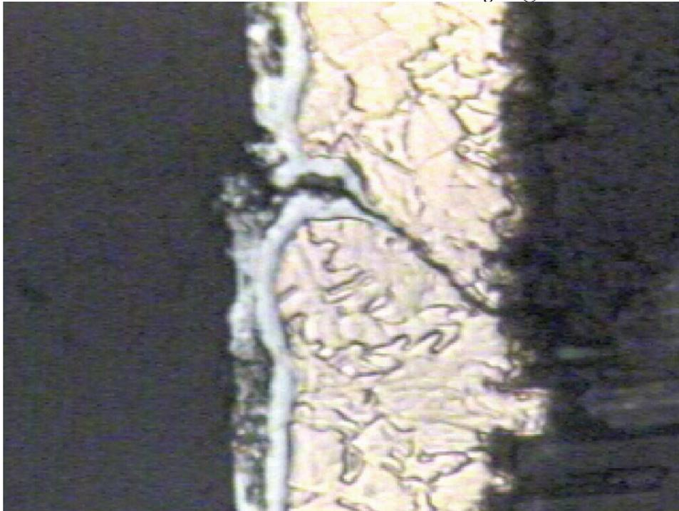
**Coupon # 0805C-5989B - Mean Cu = .0013" – 1691 Cycles – PTH Failure**
