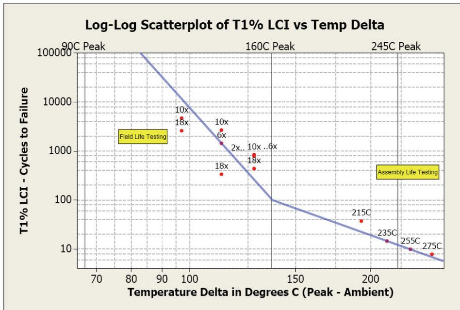
**Graph 5 – Log-log plot of T1% lower 90% two-sided confidence interval versus temperature.**
