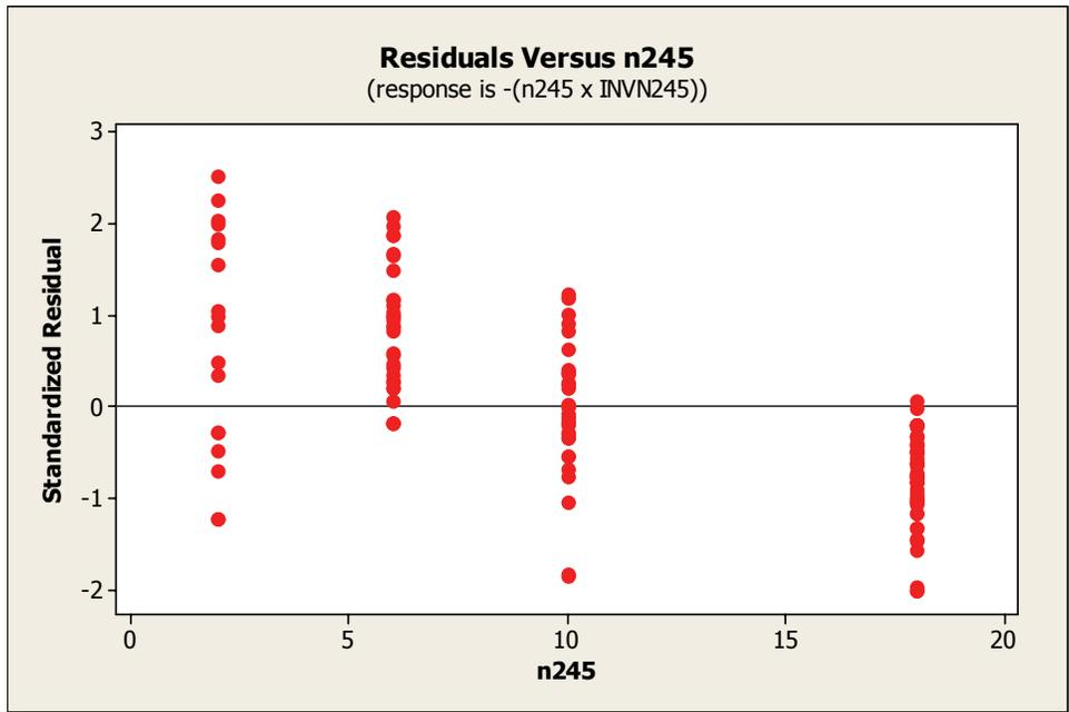
**Graph 8 – Standardized residual versus the number of preconditioning cycles shows a dip in cycles to failure with more preconditioning.**
