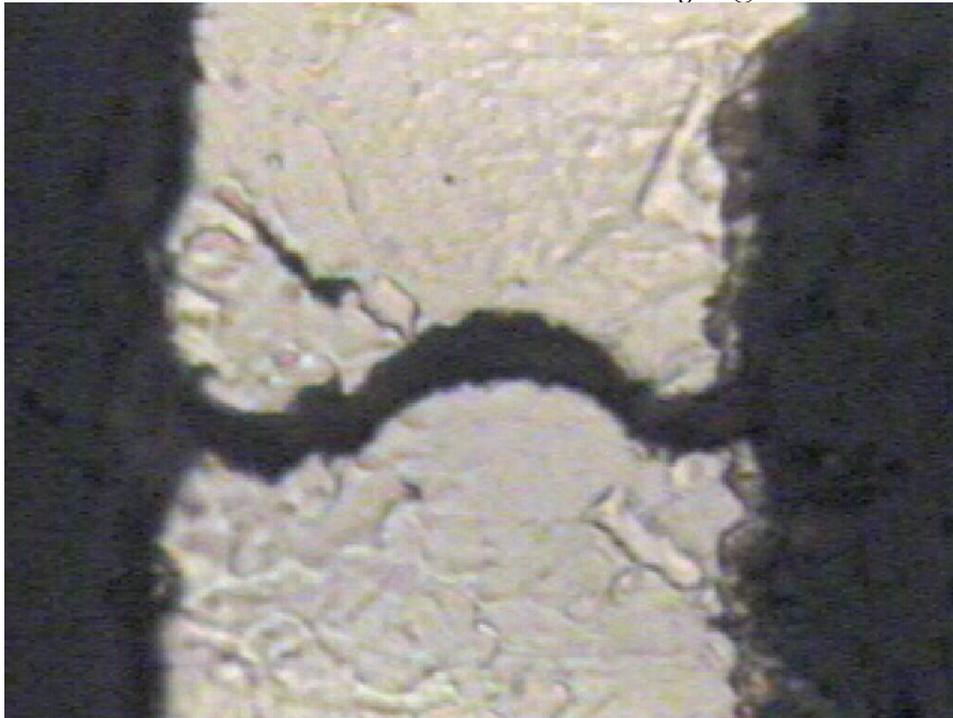
**Coupon # 0805E-5890A - Mean Cu = .0013" – 3877 Cycles – PTH Failure**
