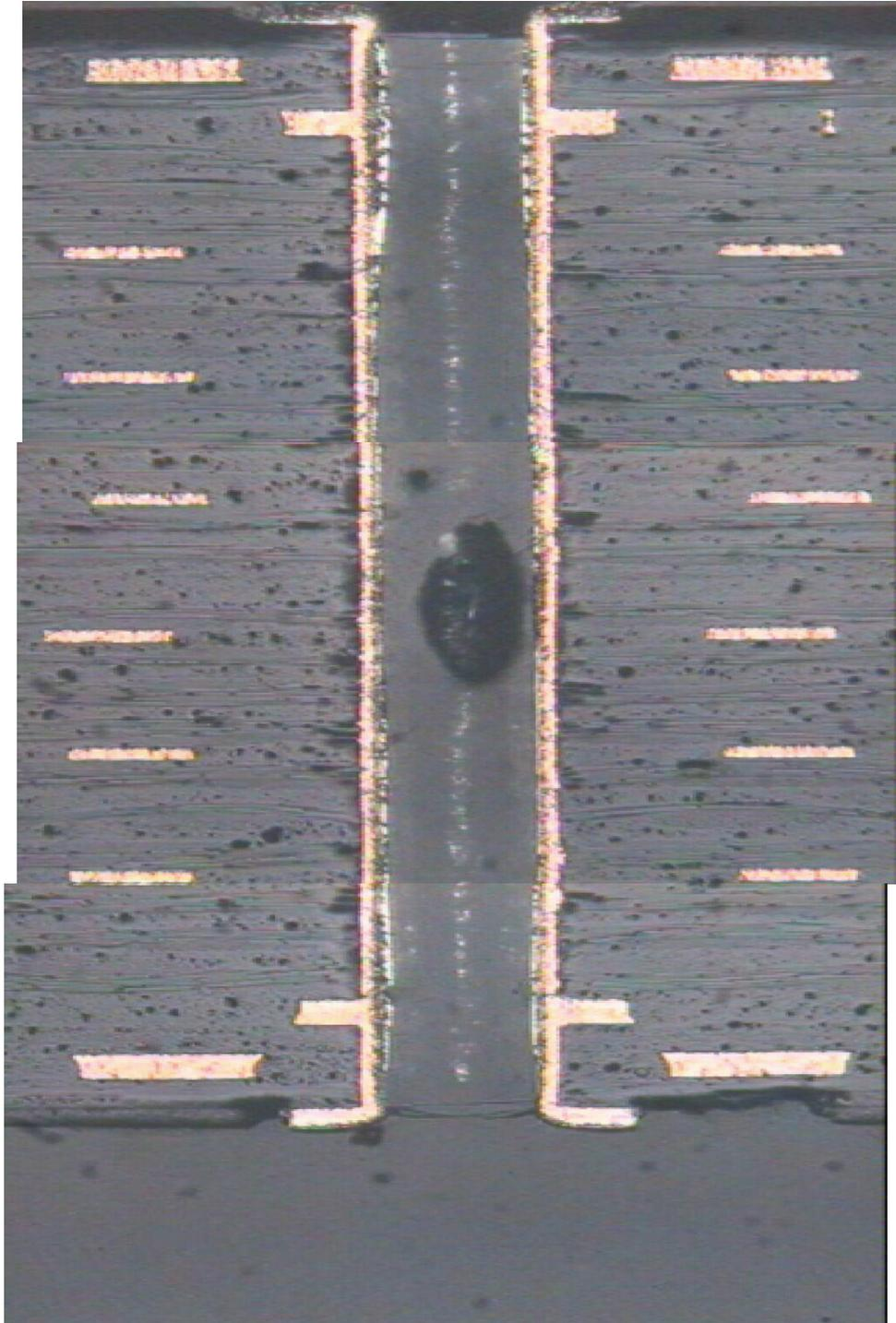
**Coupon # 0405B-5647A - Mean Cu = .0013" – 71 Cycles – PTH Failure**
