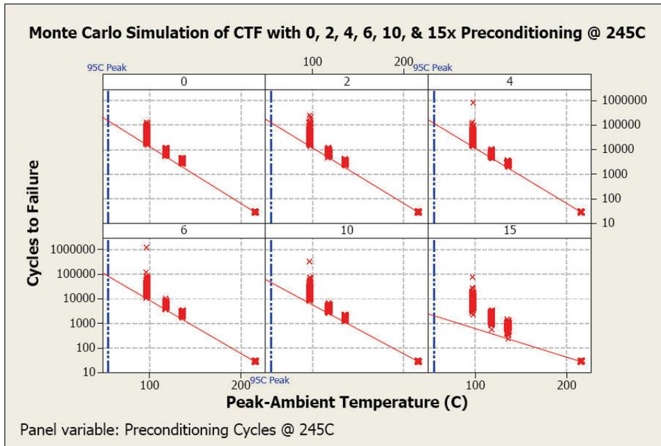
**Graph 10 – Shows CTF versus Peak-Ambient temperature as assembly preconditioning at 245°C is varied from 2 cycles to 15 cycles. Each of the four temperatures per graph contains 1000 simulated data points.**
