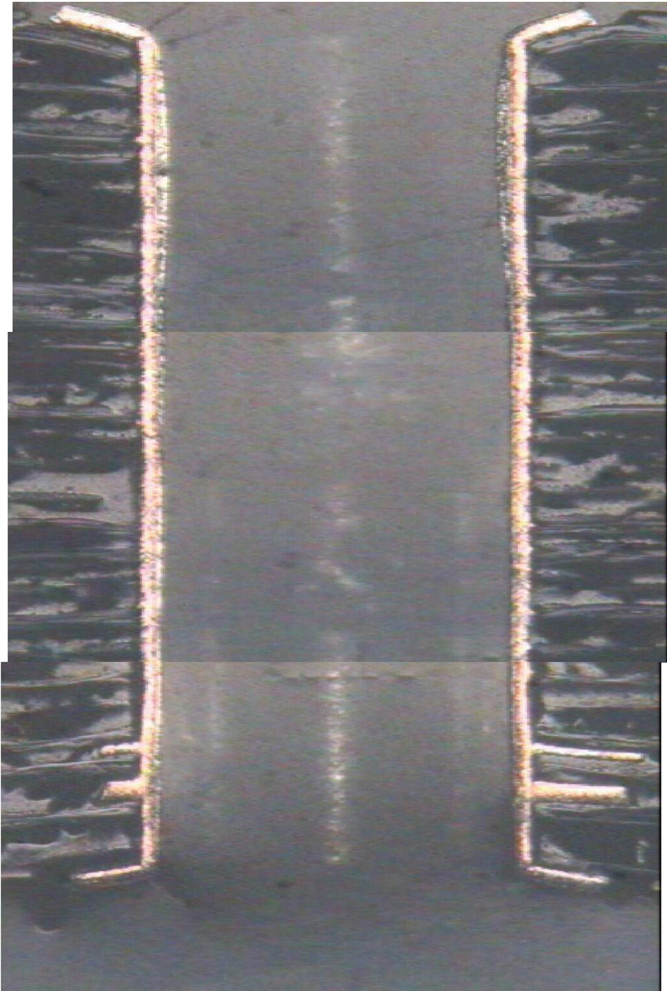
**Coupon # 0805E-5849A - Mean Cu = .0012" – 20 Cycles – Post Failure**
