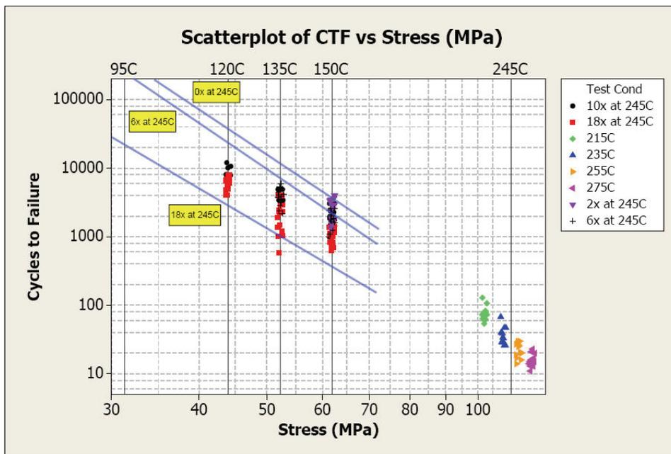
**Graph 14 – Cycle to failure versus stress scatter plot of all the raw data. The light blue lines of cycles to failure versus stress based upon Miner’s Rule.**
