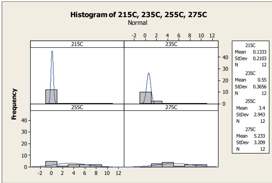
**Graph 3 – POST interconnect resistance increase (0-10%) versus IST test temperature.**
