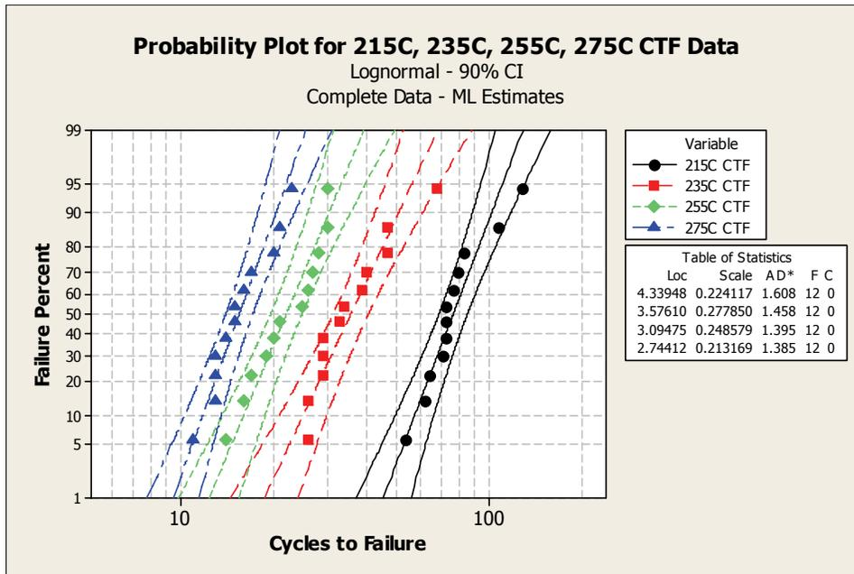
**Graph 1 – IST results from testing above Tg at four temperatures.**
