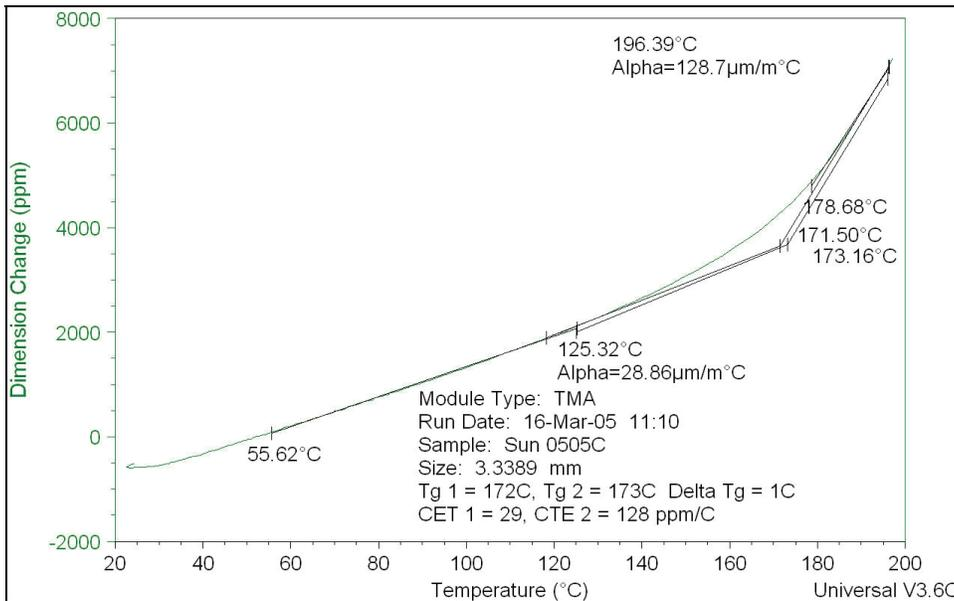
**Graph 11 – TMA plot of expansion versus temperature for board date code 0505C.**
