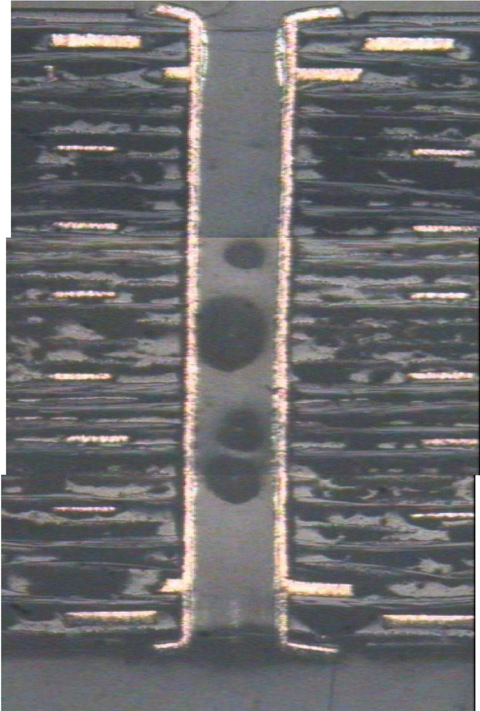
**Coupon # 0405C-5769A - Mean Cu = .0013" – 13 Cycles – PTH Failure**
