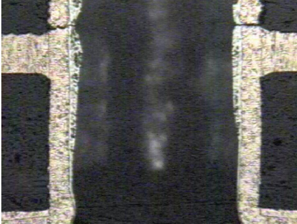
**Coupon # 0405B-5647A - Mean Cu = .0013" – 71 Cycles – PTH Failure**
