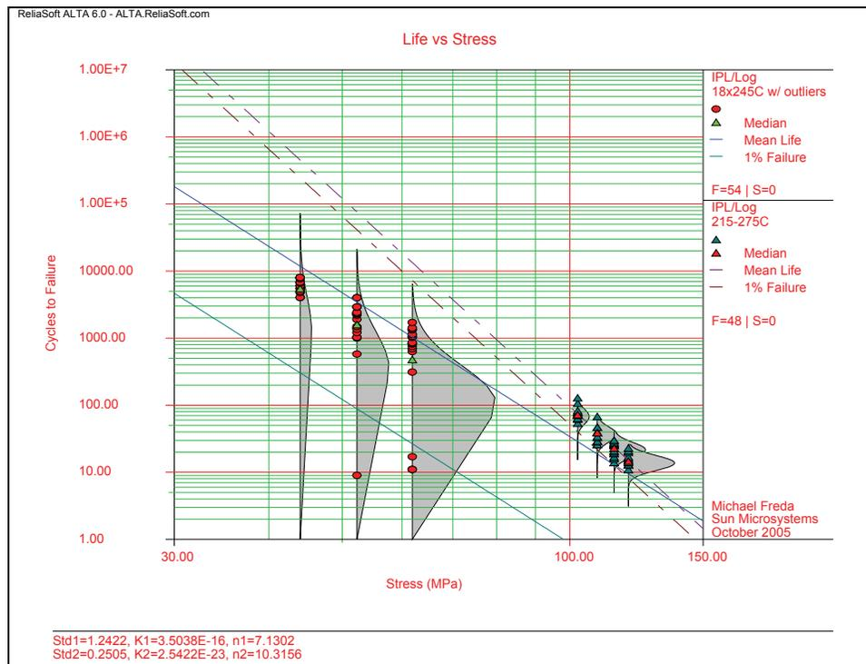
**Graph 17 – The plot uses IPL/Lognormal of stress versus cycles to failure. Separate estimates made below and above Tg due to preconditioning of 18x at 245°C below Tg. This plot includes all data points from testing with 18x preconditioning at 245°C including four outliers omitted from earlier analysis.**
