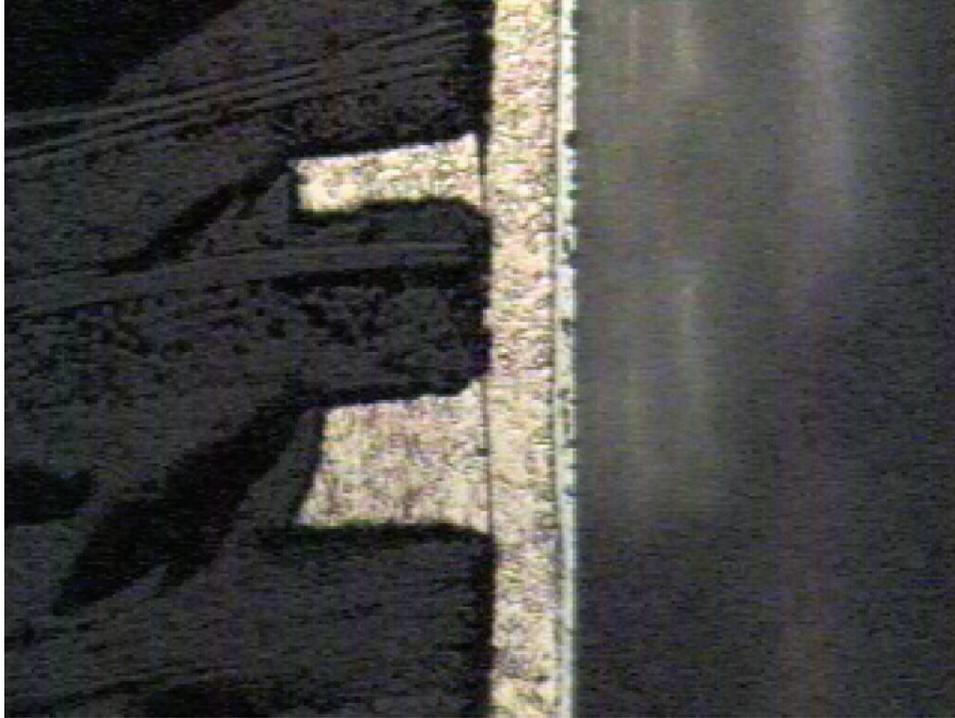
**Coupon # 0805E-5849A - Mean Cu = .0012" – 20 Cycles – Post Failure**
