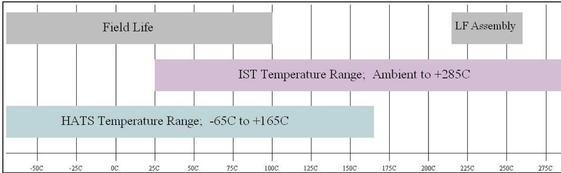
**Figure 1 – Comparison of HATS and IST test temperature ranges to Field Life and Lead-Free Assembly temperatures.**
