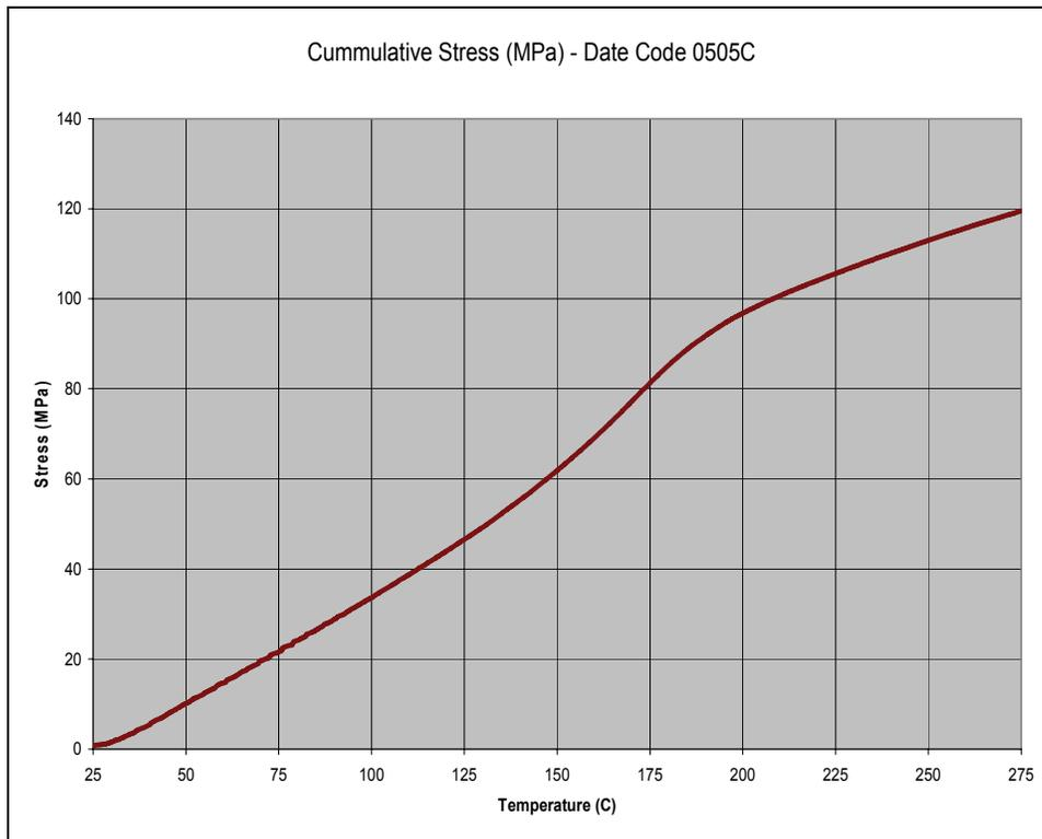
**Graph 13 – Plot of stress on copper PTH vs temperature derived from TMA and DMA.**
