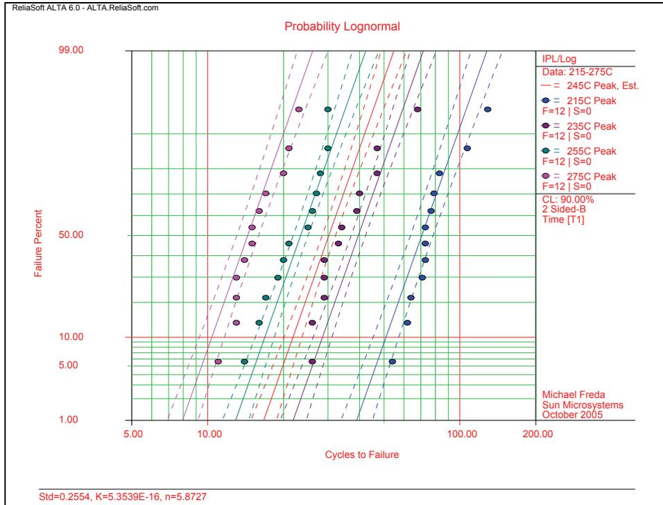
**Graph 2 – IST test results from >T<sub>g</sub> at four temperatures. Inverse Power Law relationship used to establish the best fit to the data at multiple temperatures. The RED lines show estimated CTF at 245°C.**
