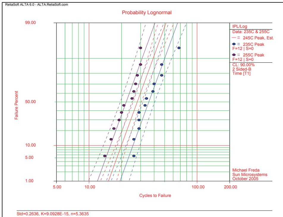
**Graph 4 – IST test results >T<sub>g</sub> at two temperatures, 235°C and 255°C. The RED lines show estimated CTF at 245°C.**
