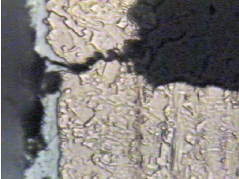
**Coupon # 0405C-5769A - Mean Cu = .0013" – 13 Cycles – PTH Failure**
