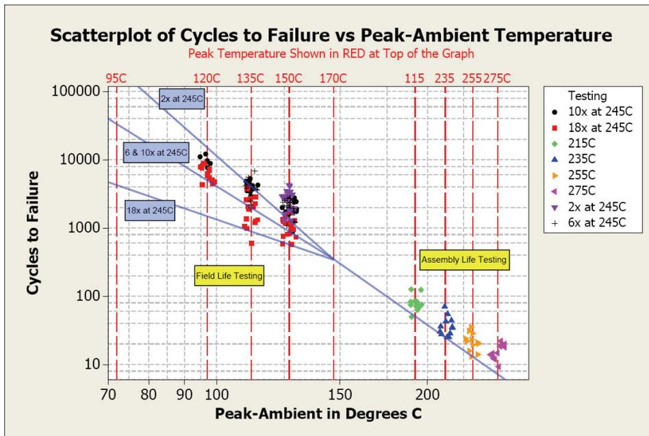
**Graph 6 – Log-log plot of all cycle to failure data versus temperature.**
