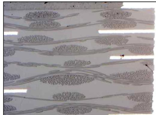
Section along the lateral direction of the IST coupon
