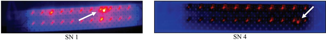
**Figure 13 – Infrared images taken when the PTH sense nets (PTH barrels) were powered. The bright spots represent the worst damage locations.**
